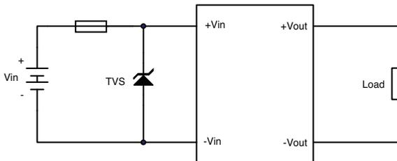
The QSB400 series converters have no internal fuse. In order to achieve maximum safety and system protection, always use an input line fuse. We recommended a 60A time delay fuse for 24Vin models, and 30A for 48Vin models. It is recommended that the circuit have a transient voltage suppressor diode TVS (24 Vin SMCJ40A; 48 Vin, SMCJ78A) across the input terminal to protect the unit against surge or spike voltage and input reverse voltage (as shown).
