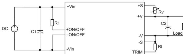
C1 = 1000  $\mu$ F / 50 V for Vin = 24 V, 330  $\mu$ F / 100 V for Vin = 48 V
