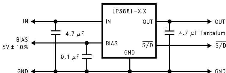
At least 4.7 µF of input and output capacitance is required for stability.
