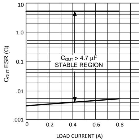
**Figure 19. Minimum ESR vs Output Load Current**
