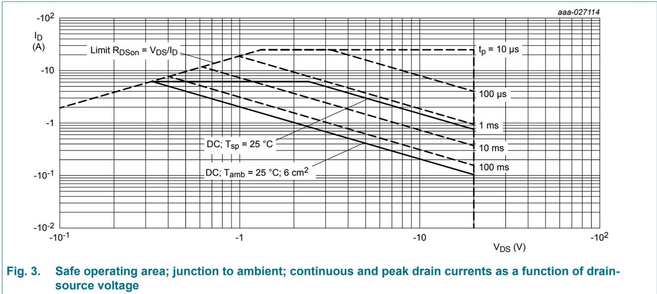
Fig. 3. Safe operating area; junction to ambient; continuous and peak drain currents as a function of drain-source voltage
