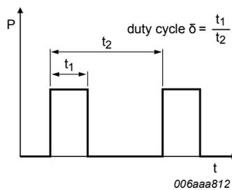
Fig. 17. Duty cycle definition
