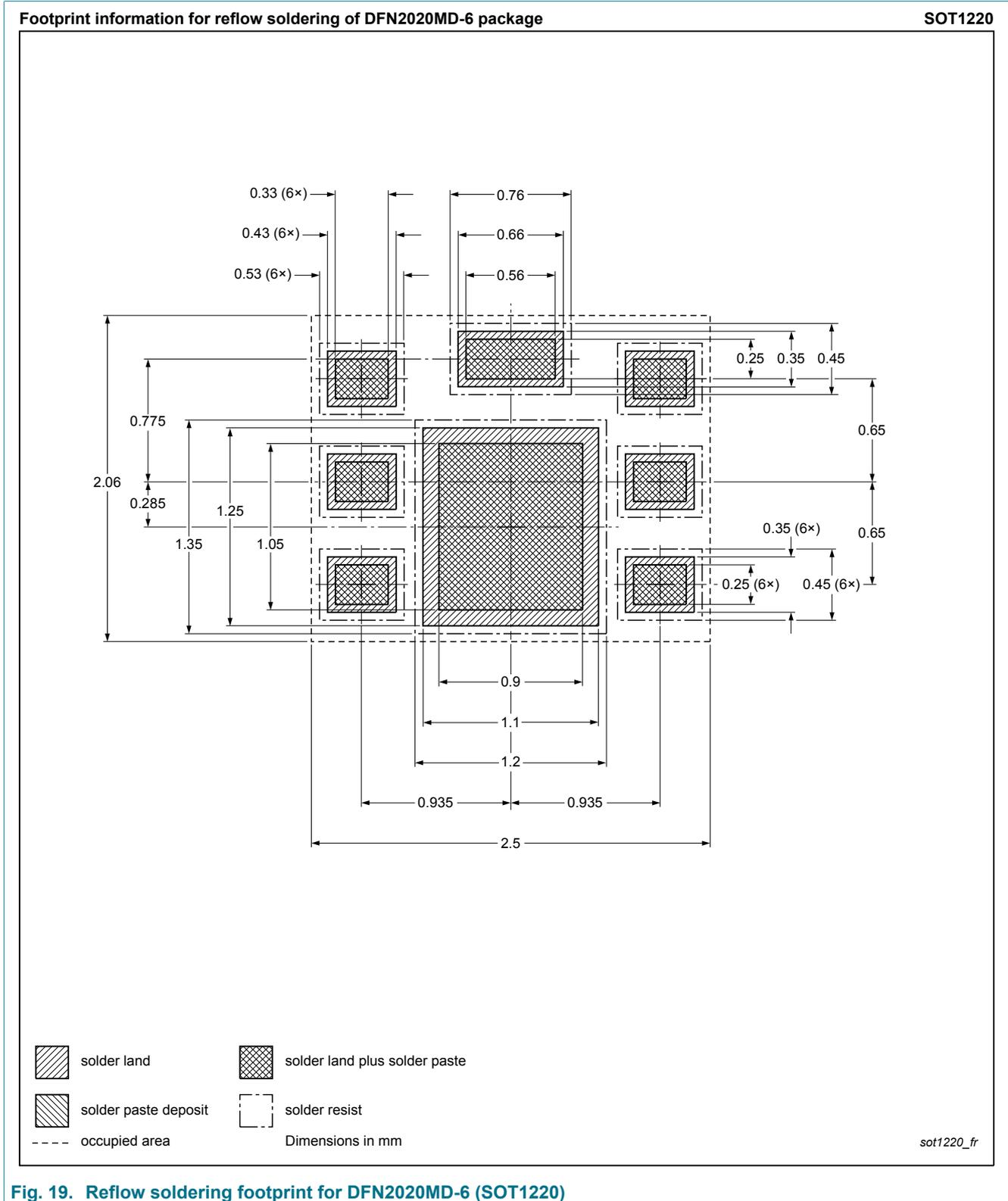
Fig. 19. Reflow soldering footprint for DFN2020MD-6 (SOT1220)
