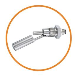
The SSF217 series are horizontally mounted switches that are fitted via 1/2"BSP thread from the outside of the tank, so does not require access to the inside of the tank.
