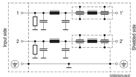
**Circuit diagram 2: 4 line filters 63A/100A with 100 dB from 150 kHz**
