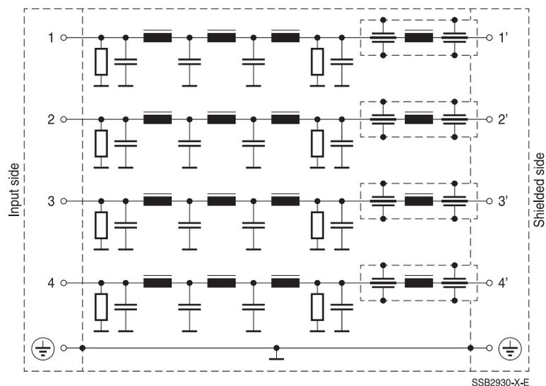
**Circuit diagram 7: 4 line filters 250A with 100 dB from 150 kHz**
