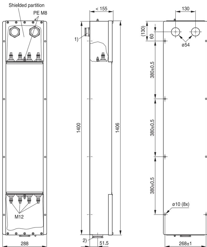
1) Cable glands PG 42\* with indented sealing ring,
