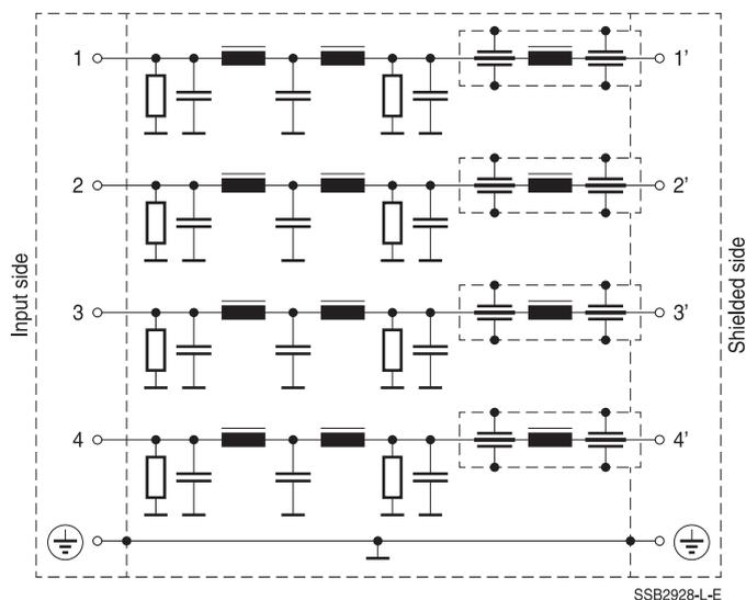
**Circuit diagram 5: 2 line filters 100A with 100 dB from 14 kHz**
