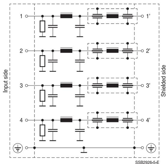
**Circuit diagram 3: 2 line filters 63A with 100 dB from 14 kHz**
