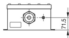
1) Cable glands PG 48\* with indented sealing ring,
