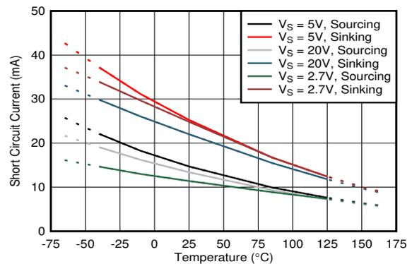
**Figure 6-22. Short-Circuit Current vs. Temperature**
