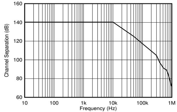
**Figure 6-44. Channel Separation vs. Frequency, Multichannel Devices**
