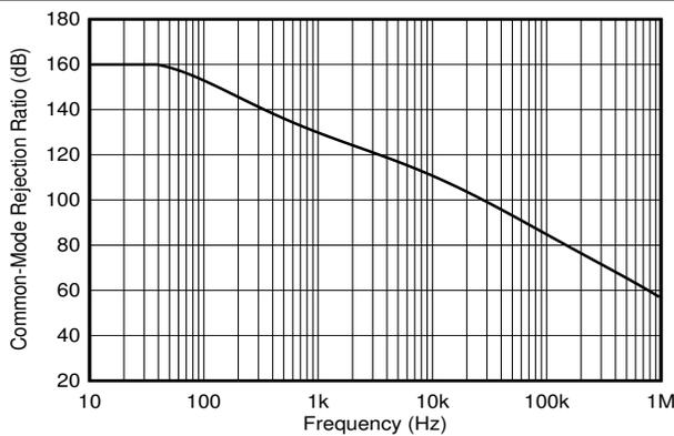
**Figure 6-9. Common-Mode Rejection Ratio vs. Frequency**
