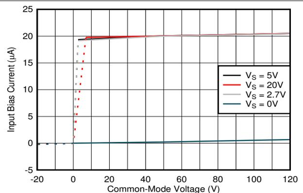
Figure 6-14. Input Bias Current vs. Common-Mode Voltage
