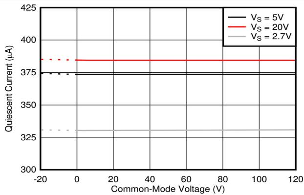
**Figure 6-37. Quiescent Current vs. Common-Mode Voltage, INA290**
