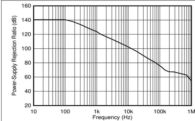
Figure 6-13. Power-Supply Rejection Ratio vs. Frequency
