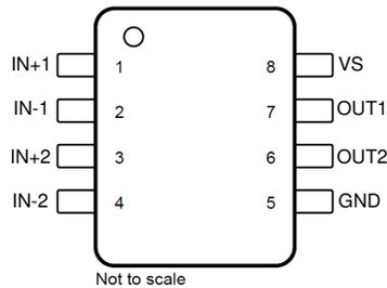
**Figure 5-2. INA2290: DGK Package 8-Pin VSSOP Top View**
