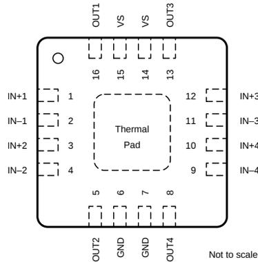
A. Thermal Pad can be left floating or connected to GND.
