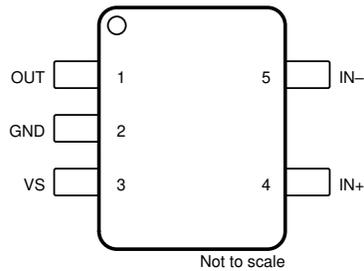
**Figure 5-1. INA290: DCK Package 5-Pin SC-70 Top View**
