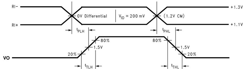
Figure 9. Receiver Propagation Delay and Transition Time Waveforms
