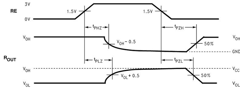
Figure 11. Receiver TRI-STATE Delay Waveforms TRI-STATE Delay Waveforms
