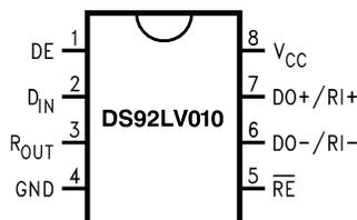
**Figure 1. SOIC Package**
