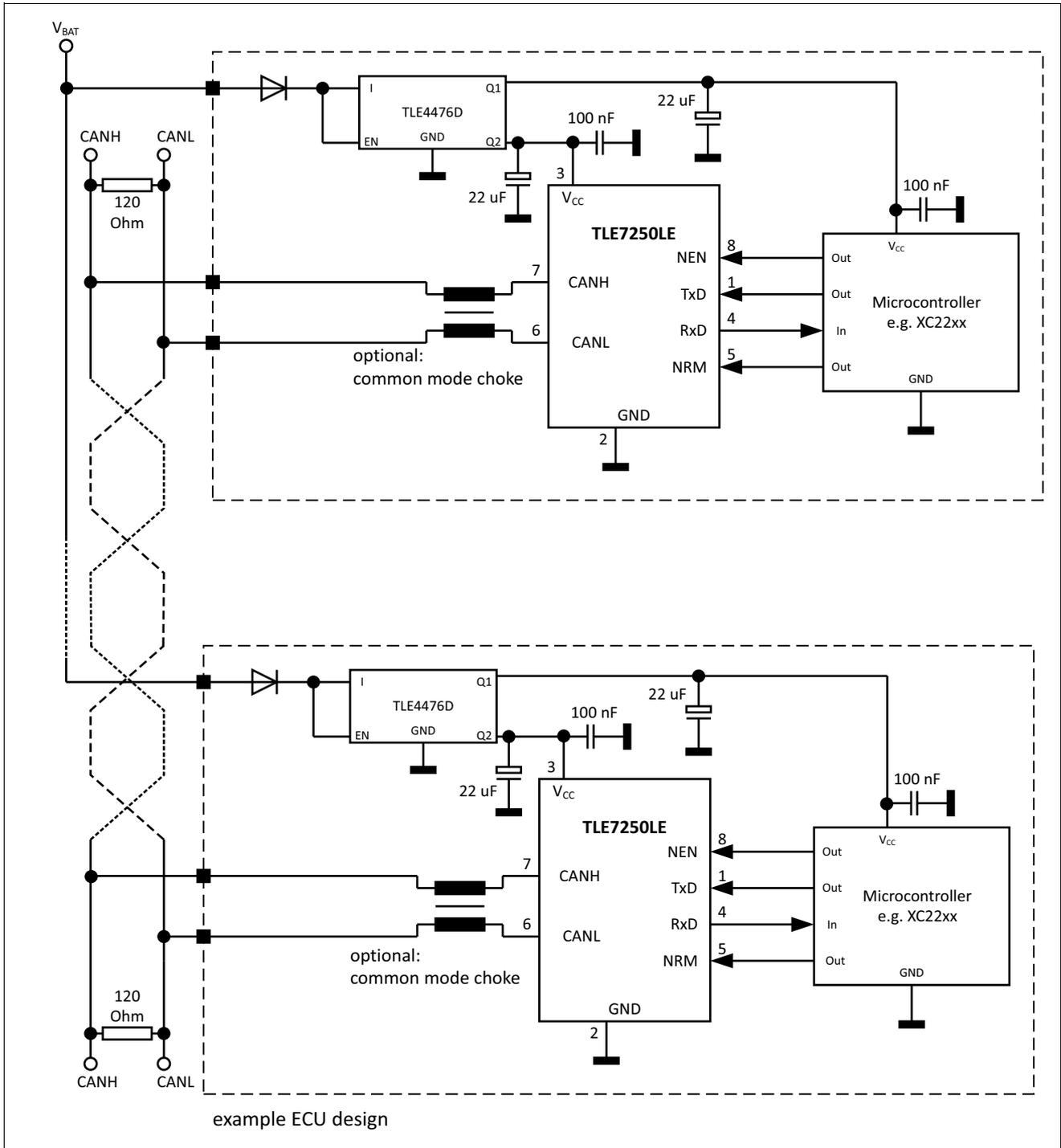
Figure 12 Application circuit
