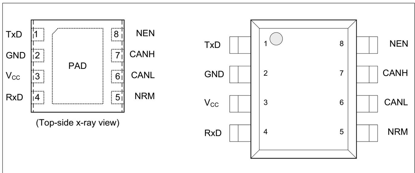
Figure 2 Pin configuration
