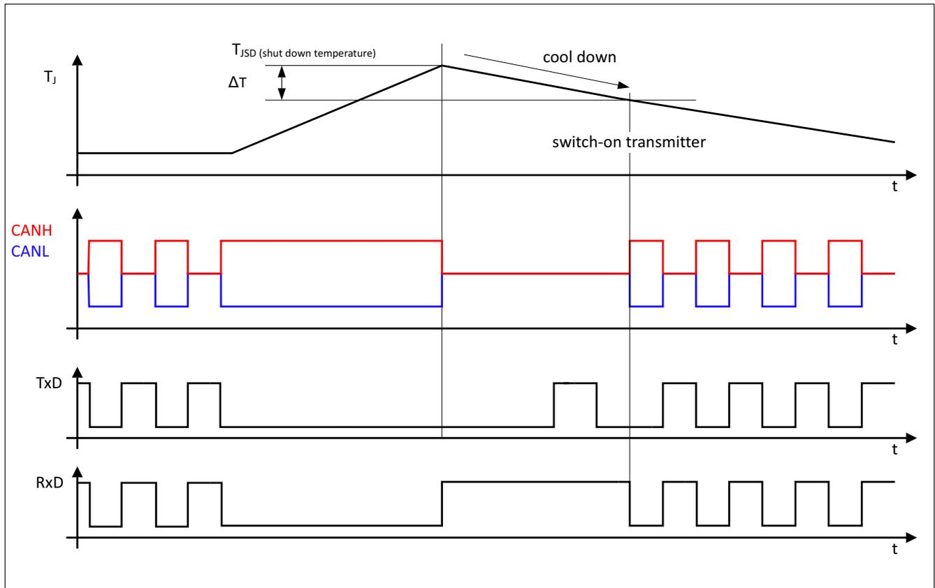
Figure 8 Overtemperature protection
