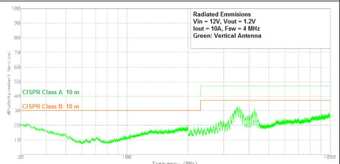
**Figure 27. Radiated Emissions 12-V Input, 1.2-V Output, 10-A Load, Vertical Antenna**
