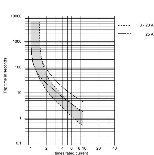
The time/current characteristic curve depends on the ambient temperature prevailing. In order to eliminate nuisance tripping, please multiply the circuit breaker current ratings by the derating factor shown below. See also section Technical information.
