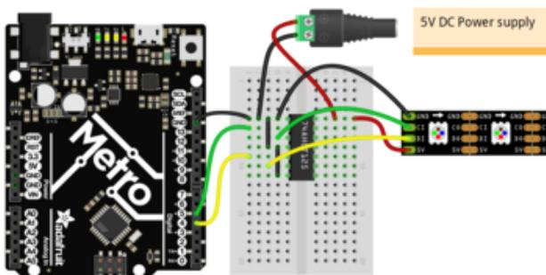
DotStars are 5 Volt devices. They may respond to 3.3V signals, but this is not a guaranteed thing. If using a 3.3V controller (Feather, Raspberry Pi, etc.), add a logic level shifter to boost 3V logic to 5V... something like a [74AHCT125](#) () on the data and clock pins.
