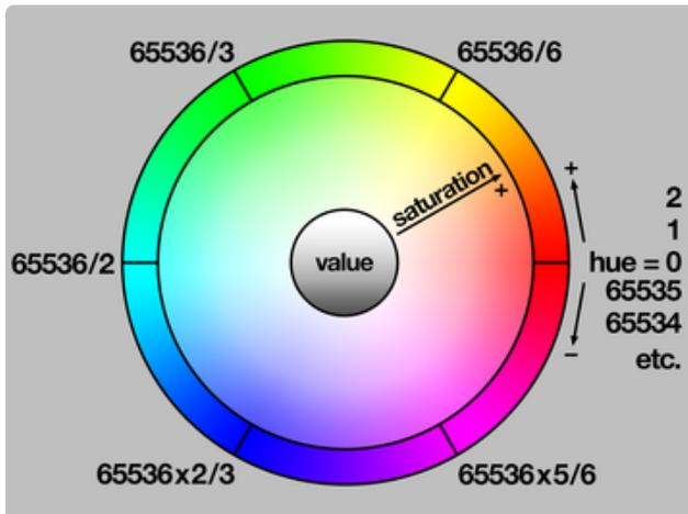
Saturation determines the intensity or purity of the color...this is an 8-bit number ranging from 0 (no saturation, just grayscale) to 255 (maximum saturation, pure hue). In the middle, you'll start to get sort of pastel tones.
