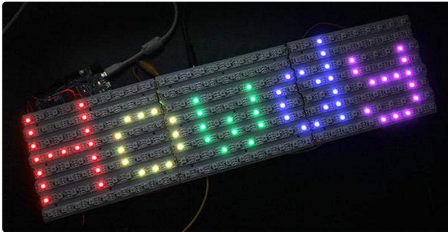
If you need a size or shape of DotStar matrix that's not offered here, it's possible to create your own using sections of DotStar strip!
