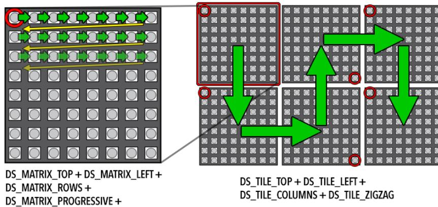
Tiles don't need to be square! The above is just one possible layout. The display shown at the top of this page is three 10x8 tiles assembled from DotStar strip.
