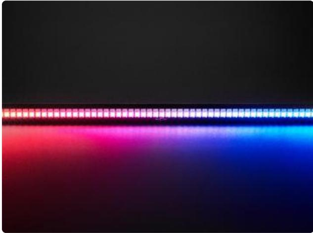
Another linear form factor similar to a strip, but this one is not flexible. It features 128 tiny DotStar LEDs packed into a 400 millimeter bar with wires at each end with 4-pin JST connectors.
