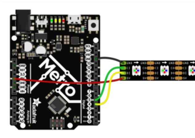
Connect the strip 5V pin to the board 5V
