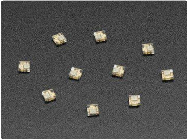
Tiny surface-mount “2020” (2.0 millimeters square) DotStars are available in RGB (no pure white option):
