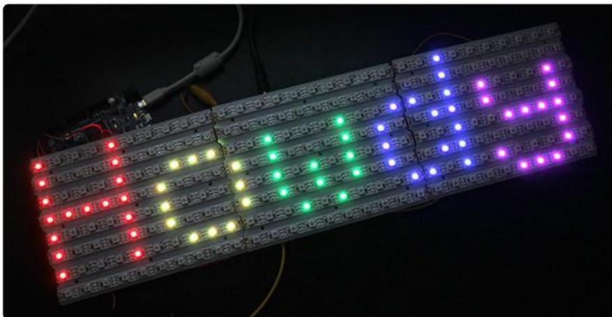
The `Adafruit_DotStarMatrix` library builds upon `Adafruit_DotStar` to create two-dimensional graphic displays using DotStar LEDs. You can then easily draw shapes, text and animation without having to calculate every X/Y pixel position. Small DotStar matrices are available in the shop. Larger displays can be formed using sections of DotStar strip, as shown above.
