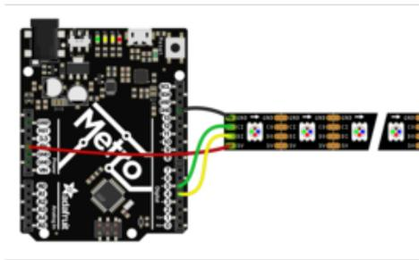
The simplest wiring is if you can power the strip off of the microcontroller board itself. This is fine for small projects (one or two dozen DotStars max) because we don't light up a lot of LEDs at once.
