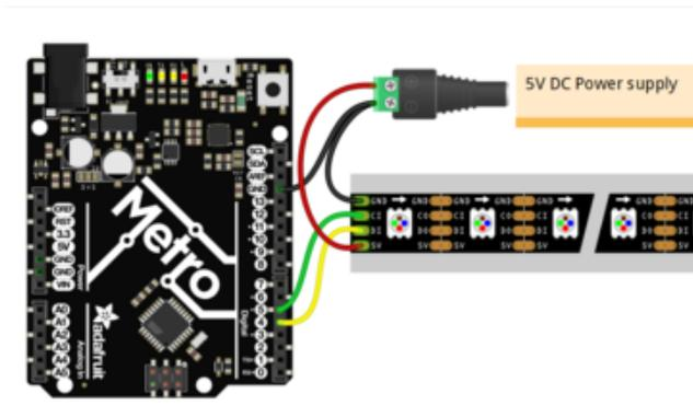
Connect the strip 5V pin to the power adapter 5V
