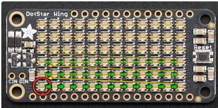
We refer to this layout as row major and progressive. Row major means the pixels are arranged in horizontal lines (the opposite, in vertical lines, is column major). Progressive means each row proceeds in the same direction. Some matrices will reverse direction on each row, as it can be easier to wire that way. We call that a zigzag layout.
