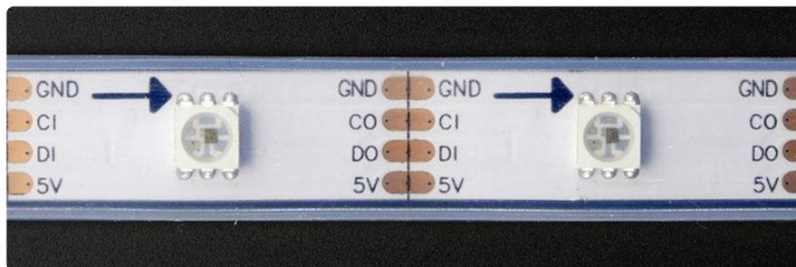
First, look for arrows printed along the strip next to each LED. These show the direction of data moving down the strip...your microcontroller connects at the originating (“in”) end, the arrows point toward the “out” end. (In the photo above, our microcontroller would be located off the left side.)
