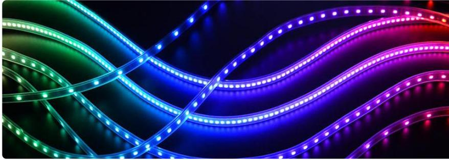
NeoPixel LEDs are the bee's knees, but in a few scenarios they come up short... connecting odd microcontrollers that can't match their strict timing, or fast-moving persistence-of-vision displays. Adafruit DotStar LEDs deliver high speed PWM and an easy-to-drive two-wire interface, bridging the gaps in the spectrum of awesome.
