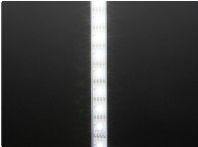
A recent addition is White DotStar strips. Rather than red, green and blue, these contain three identical white LED elements — either “cool” or “warm” white. For monochrome applications, white DotStars are more “true” and pleasing to the eye than white mixed from red+green+blue. Like the RGB strips, they’re available in different pixel densities.
