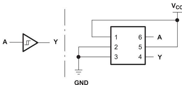
Figure 6. Noninverted Buffer
