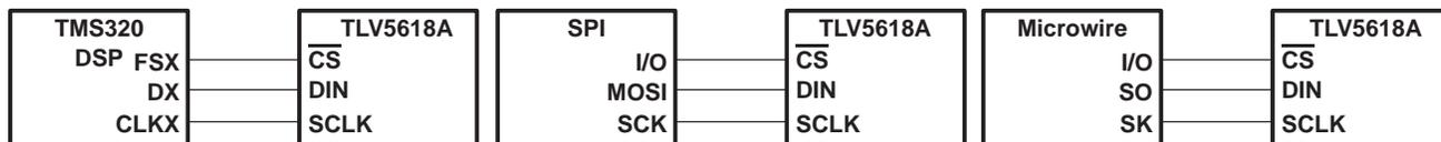
**Figure 12. Three-Wire Interface**
