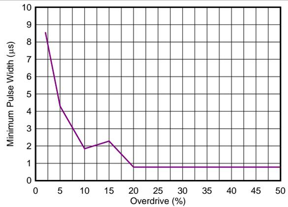
$V_{DD} = 24\text{ V}$ , minimum pulse duration required to trigger output high-to-low transition, SENSE = negative spike below  $V_{IT-}$ .
