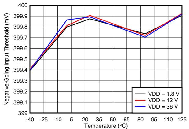
Figure 5. SENSE Negative Input Threshold Voltage ( $V_{IT-}$ ) vs Temperature
