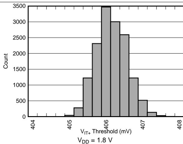
Figure 6. SENSE Positive Input Threshold Voltage ( $V_{IT+}$ ) Distribution
