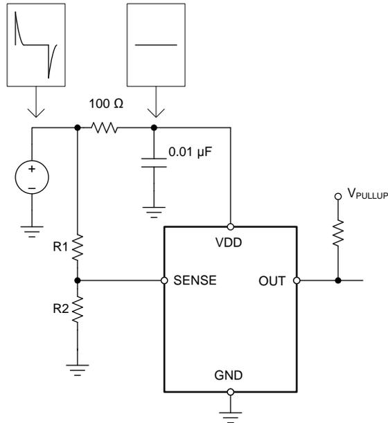
**Figure 17. Using a RC Filter to Remove High-Frequency Disturbances on V<sub>DD</sub>**
