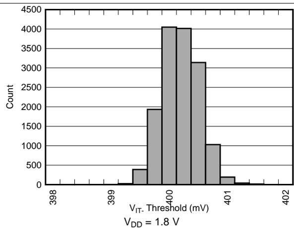
Figure 7. SENSE Negative Input Threshold Voltage ( $V_{IT-}$ ) Distribution
