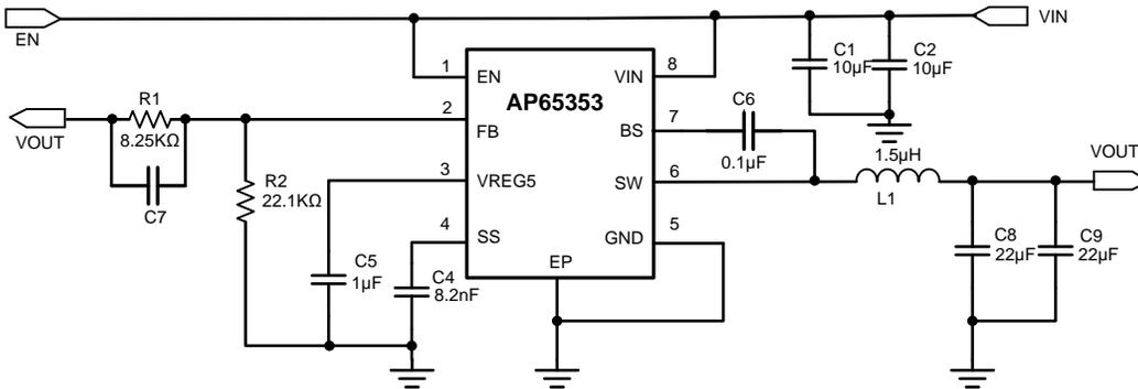
**Figure 3 Typical Application of AP65353 Evaluation Board**
