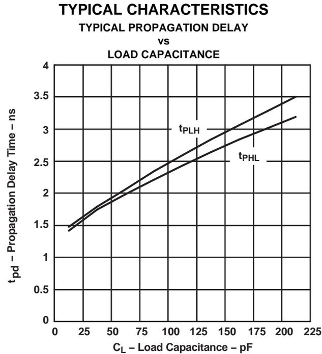
NOTE: This graph is included as an aid to the system designers. Total circuit delay varies with load capacitance. The total delay is the sum of the delay due to external capacitance and the intrinsic delay of the device. Intrinsic delay is listed in the table above as the 0 pF load condition. The incremental increase in delay between the 0 pF load condition and the actual total load capacitance represents the extrinsic, or external delay contributed by the load.
