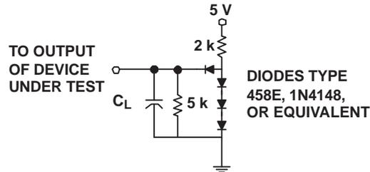
$C_L$  includes test-fixture and probe capacitance.
