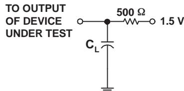
$C_L$  includes test-fixture and probe capacitance.
