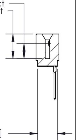
726 Series Ultra-Mate Card Edge Connector - Press Fit
