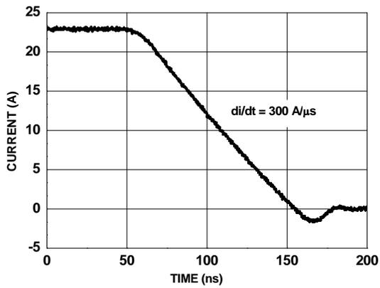
Figure 14. FDMS2510SDC SyncFET body diode reverse recovery characteristic
