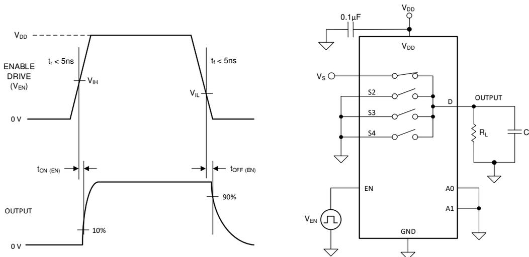
Figure 12. Turn-On and Turn-Off Time Measurement Setup
