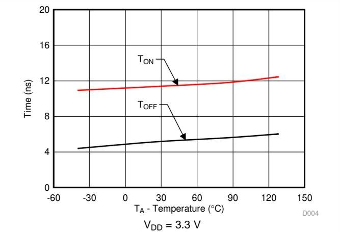
Figure 4.  $T_{ON}$  (EN) and  $T_{OFF}$  (EN) vs Temperature
