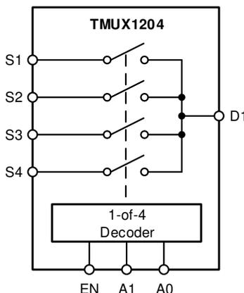
**Figure 17. TMUX1204 Functional Block Diagrams**
