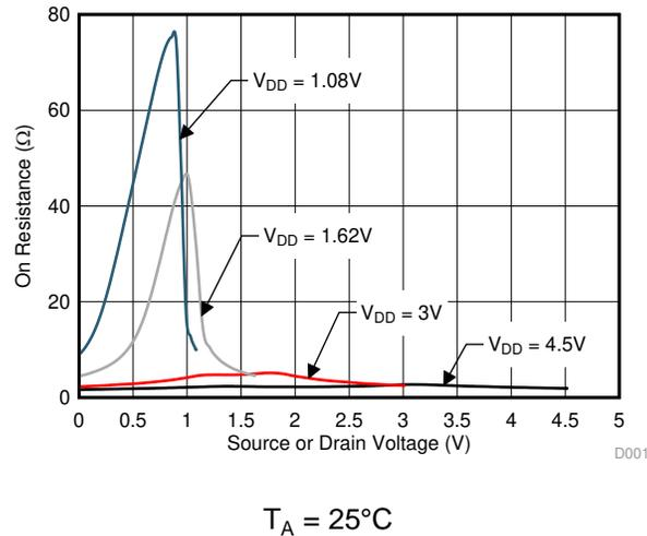
**Figure 19. On-Resistance vs Source or Drain Voltage**
