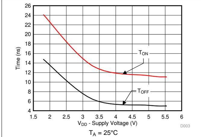
Figure 3.  $T_{ON}$  (EN) and  $T_{OFF}$  (EN) vs Supply Voltage
