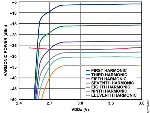
Figure 6. RF Output Harmonic Content vs.  $V_{DDx}$
