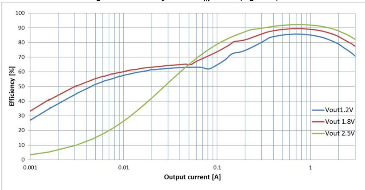
Figure 15. Load regulation ( $V_{IN} = 4\text{ V}$ )
