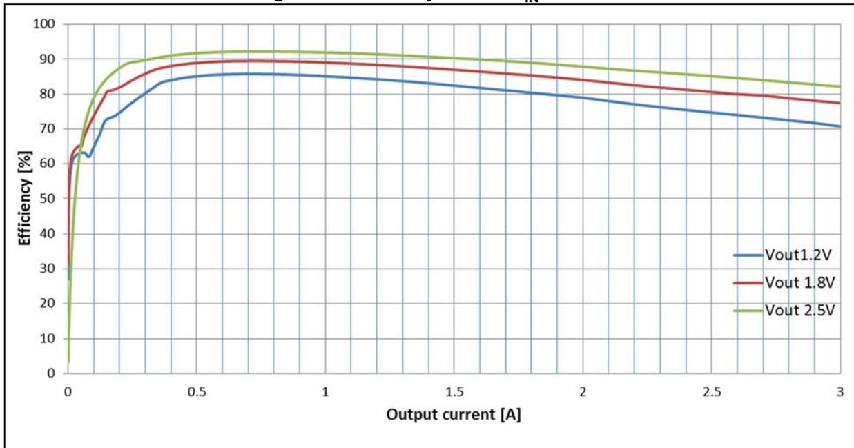
Figure 14. Efficiency curves:  $V_{IN} = 4.0\text{ V}$  (log scale)
