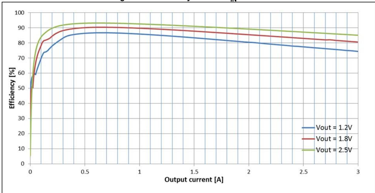
Figure 17. Efficiency curves:  $V_{IN} = 3.3\text{ V}$  (log scale)
