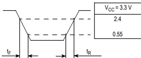
**Figure 15. Output Transition Time Test Reference**
