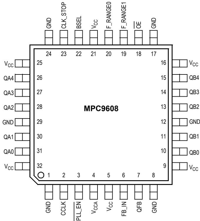
Figure 2. MPC9608 32-Lead Package Pinout (Top View)
