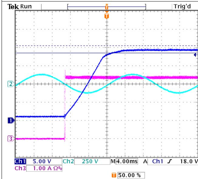
Figure 51. Output Rise-Time, 90-V<sub>AC</sub>, 3.35-A CC Load
