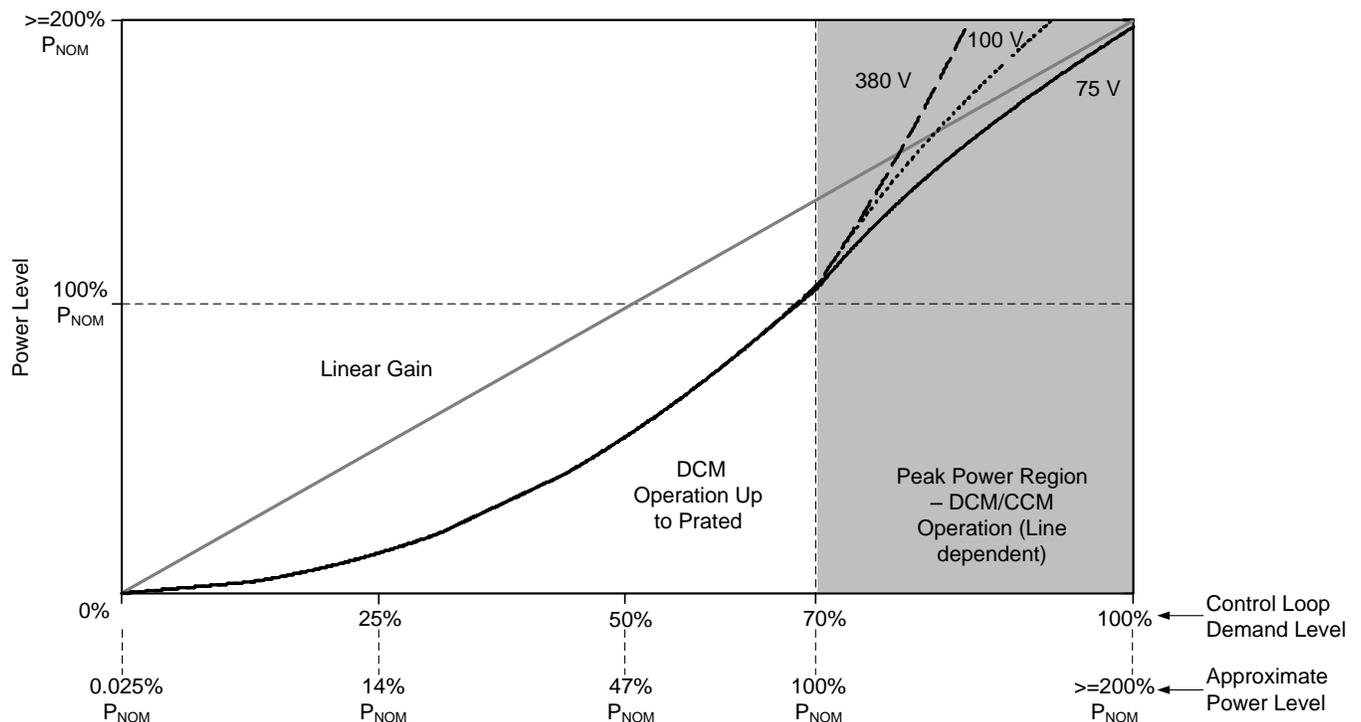
Figure 42. Modulator Gain Curves vs Bulk Capacitor Voltage
