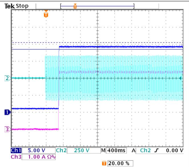
Figure 50. Start-Up from 230-V<sub>AC</sub>, 3.35-A CC Load
