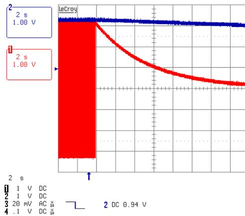
**Figure 20. X-Capacitor Decay Rate Without Active Discharge
