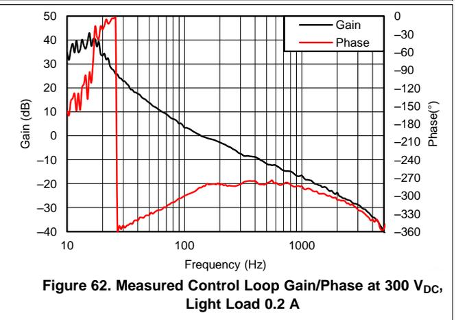
Figure 62. Measured Control Loop Gain/Phase at 300 V<sub>DC</sub>, Light Load 0.2 A
