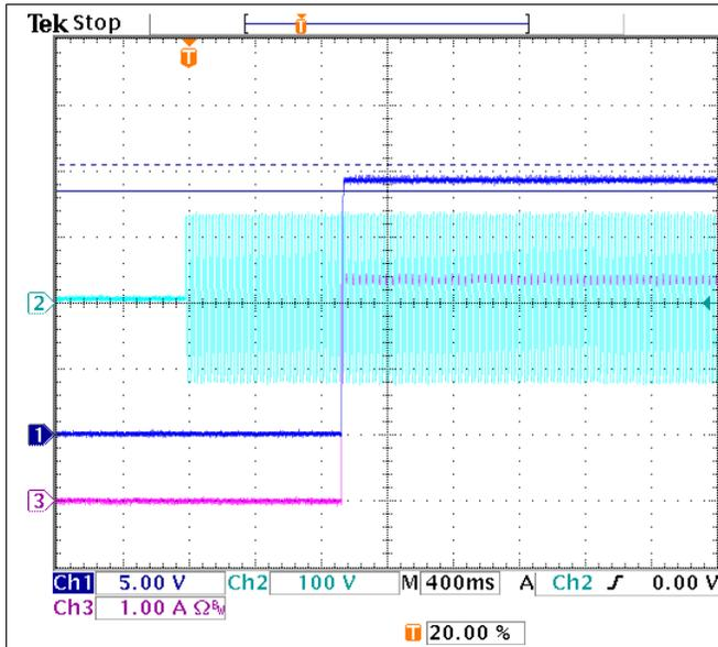
Figure 49. Start-Up from 90-V<sub>AC</sub>, 3.35-A CC Load
