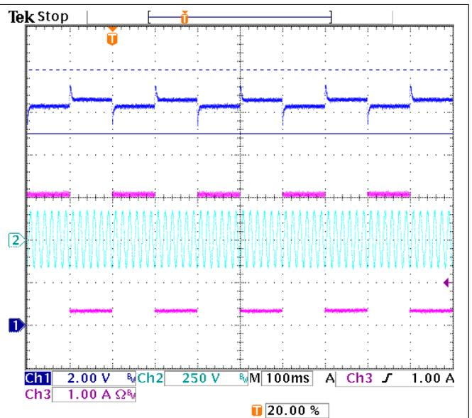
Figure 60. Transient Step 10% to 90% Load, 115 V<sub>AC</sub>
