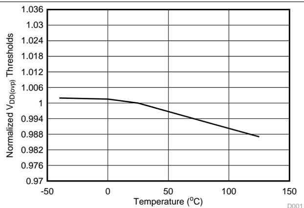
Figure 6. Normalized  $V_{DD(ovp)}$  Threshold vs. Temperature
