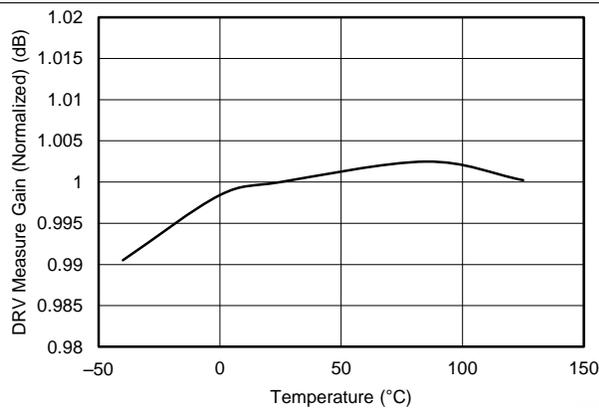
Figure 11. DRV Programming Current Measure vs. Temperature
