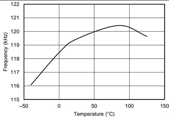
Figure 9. F<sub>SW(max)</sub> vs. Temperature
