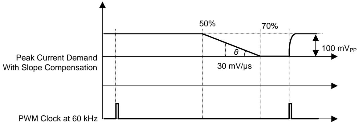
**Figure 31. Peak Current Demand with Slope Compensating Downslope**
