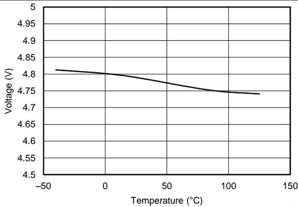
Figure 7. V<sub>DD(reset)</sub> Threshold vs. Temperature
