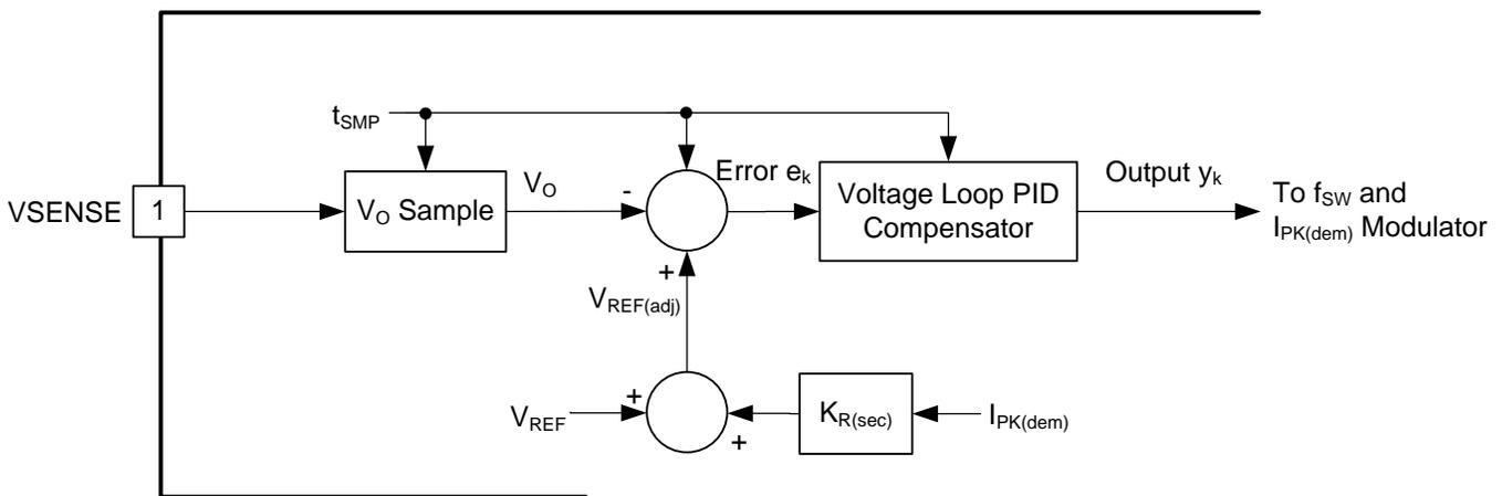
Figure 29. Digital Voltage Control Loop Simplified Block Diagram
