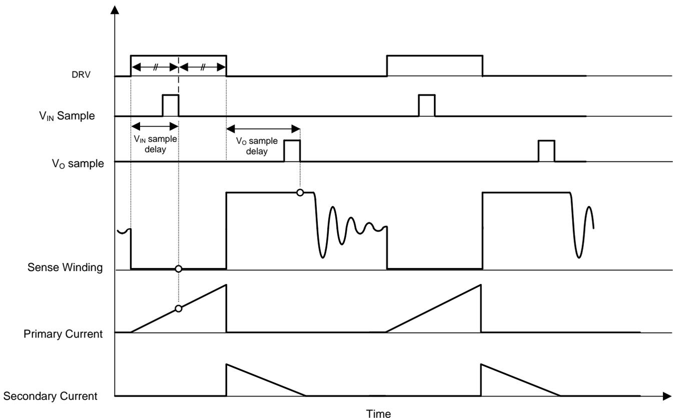
Figure 26. V<sub>IN</sub> and V<sub>OUT</sub> Sample Trigger Timing
