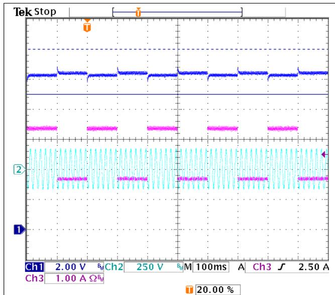
Figure 59. Transient Step 50% to 100% Load, 115 V<sub>AC</sub>
