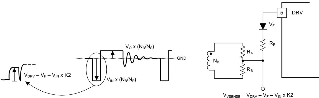
Figure 23. Line Input Sense by Offsetting the Negative Swing on the Sense Winding
