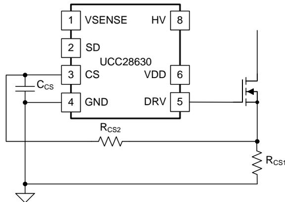
Figure 30. Primary-Side Current Sensing
