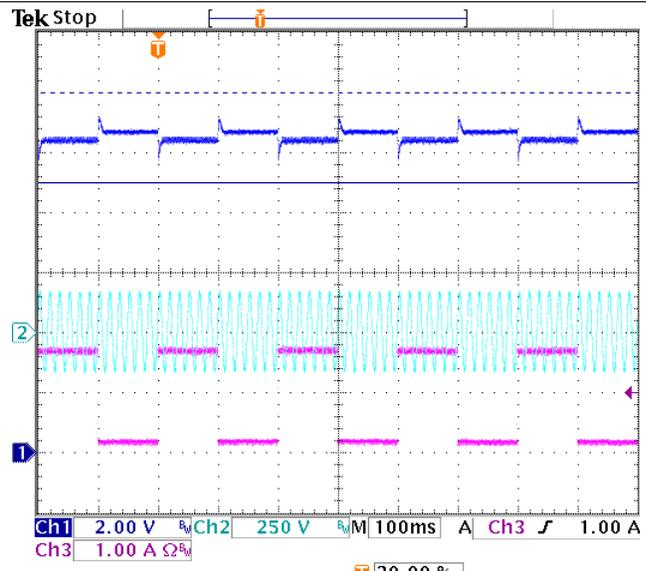
Figure 58. Transient Step 5% to 50% Load, 115 VAc
