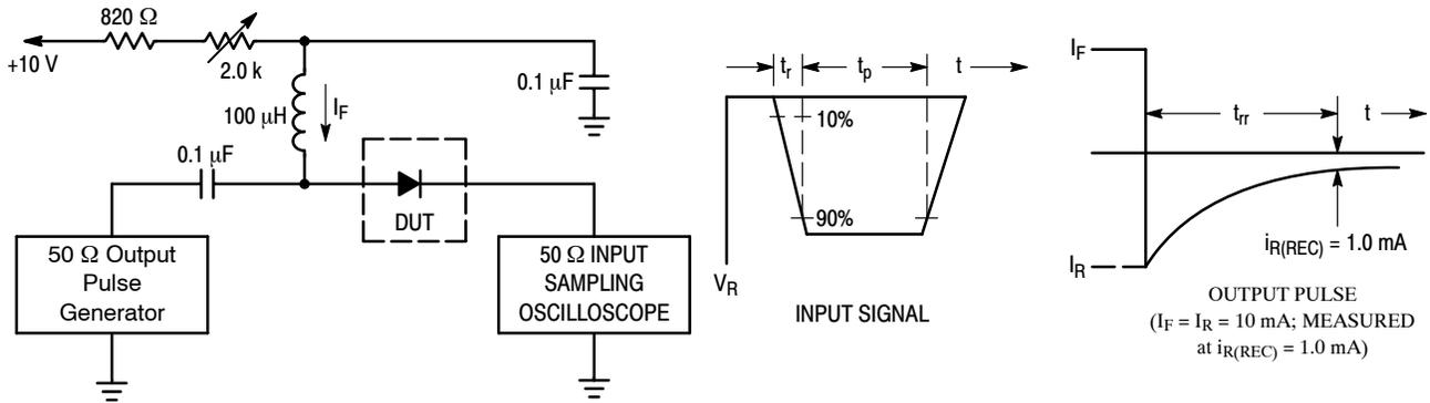
1. A 2.0 k $\Omega$  variable resistor adjusted for a Forward Current ( $I_F$ ) of 10 mA.
