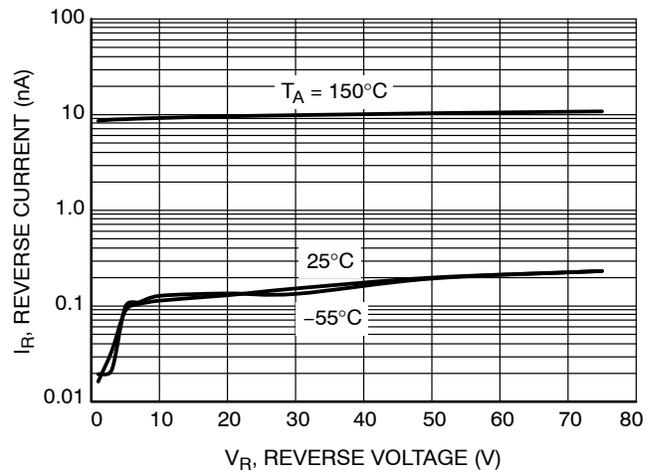
Figure 3. Leakage Current
