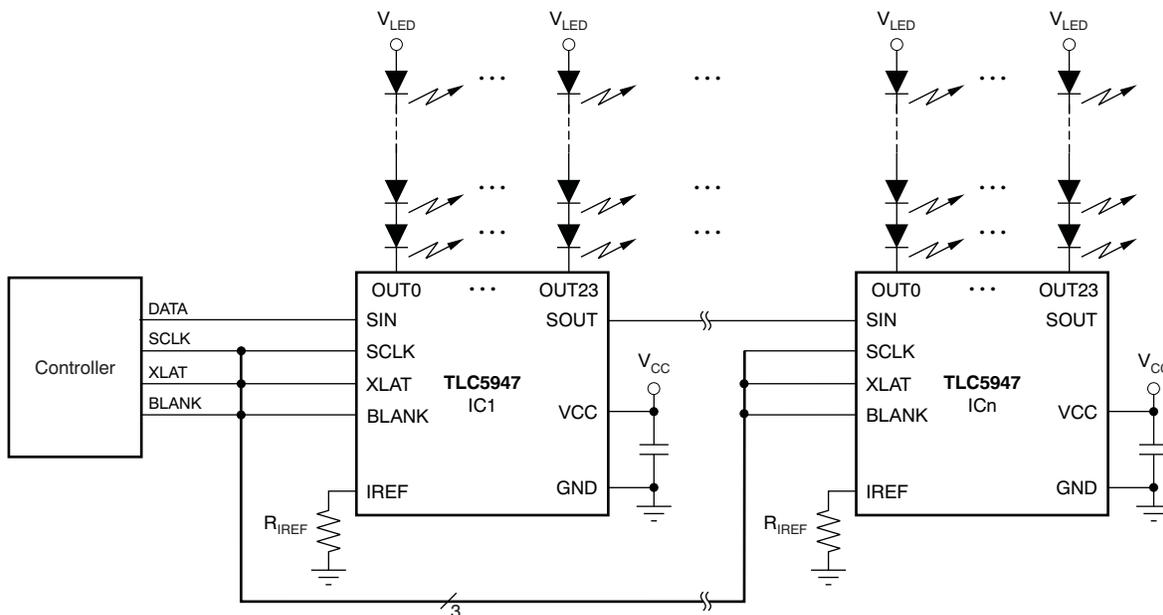
Figure 23. Typical Application Circuit (Multiple Daisy Chained TLC5947s)
