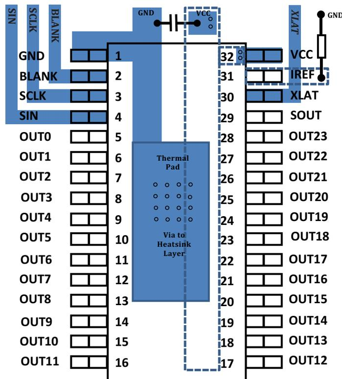
Figure 26. Layout Schematic
