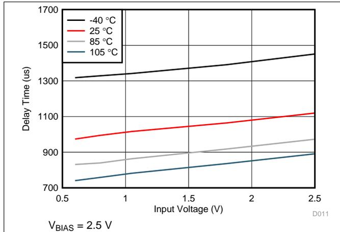
Figure 11. Delay Time vs Input Voltage
