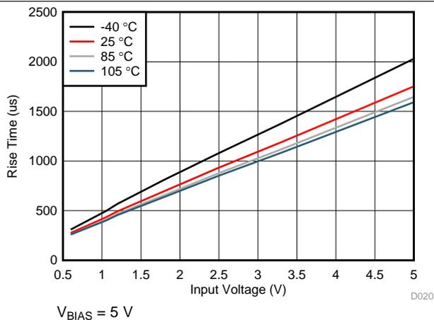
Figure 20. Rise Time vs Input Voltage
