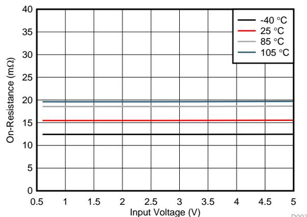
$V_{BIAS} = 5\text{ V}$ ,  $I_{VOUT} = -200\text{ mA}$
