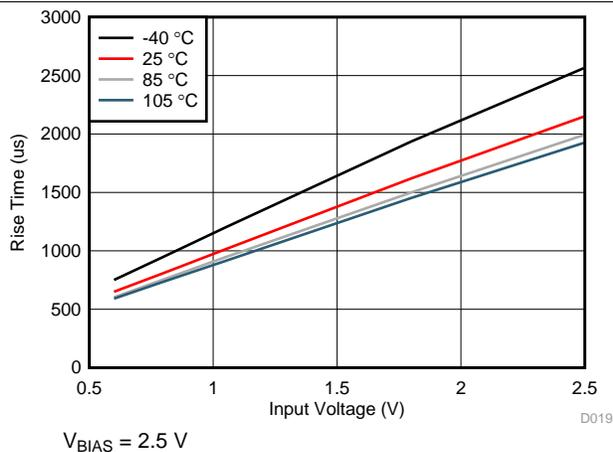
Figure 19. Rise Time vs Input Voltage
