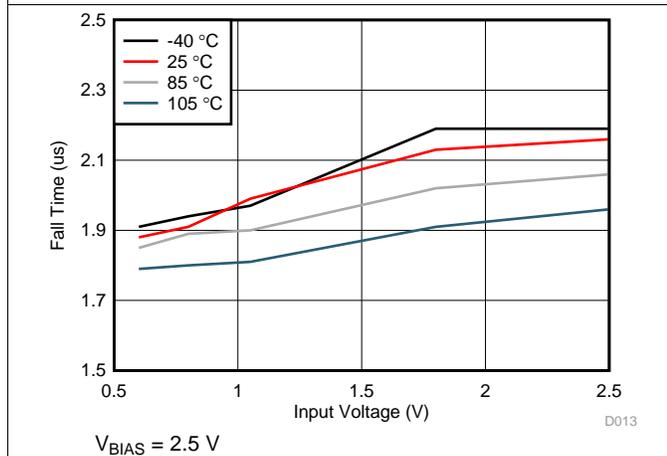
Figure 13. Fall Time vs Input Voltage
