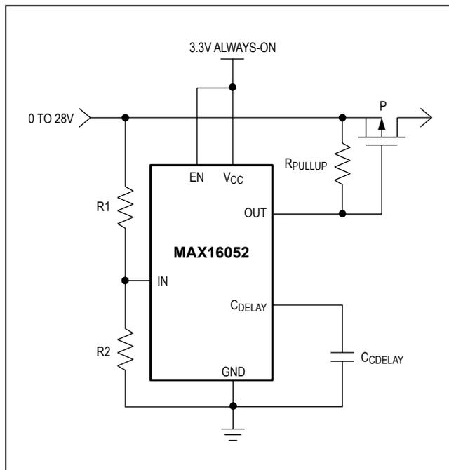
Figure 4. Overvoltage Protection
