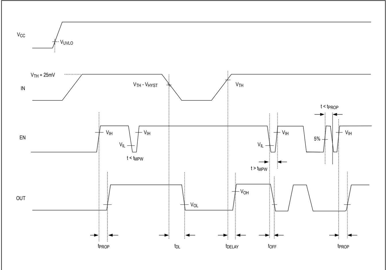
Figure 1. MAX16052/MAX16053 Timing Diagram ( $C_{DELAY} = 0$ )
