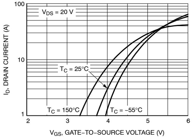
Figure 2. Transfer Characteristics
