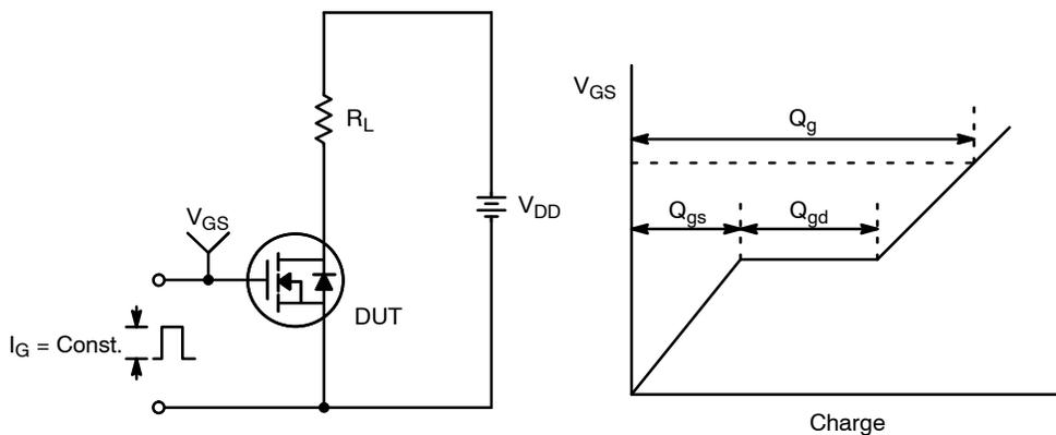
Figure 13. Gate Charge Test Circuit & Waveform
