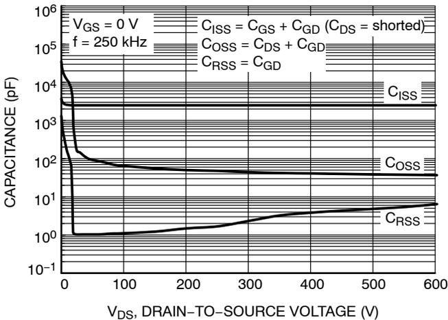
Figure 5. Capacitance Characteristics
