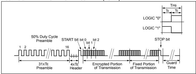
FIGURE 9-7: MANCHESTER PREAMBLE/HEADER FORMAT (MOD=1)
