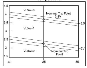
If the supply voltage drops below the low voltage trip point, the LED output will be toggled at approximately 1Hz during the transmission.
