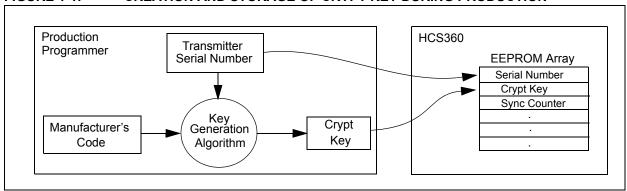
The 16-bit synchronization counter is the basis behind the transmitted code word changing for each transmission; it increments each time a button is pressed. Due to the code hopping algorithm's complexity, each increment of the synchronization value results in greater than 50% of the bits changing in the transmitted code word.
