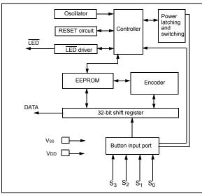
The HCS360 combines a 32-bit hopping code generated by a nonlinear encryption algorithm, with a 28/32-bit serial number and 7/3 status bits to create a 67-bit transmission stream.
