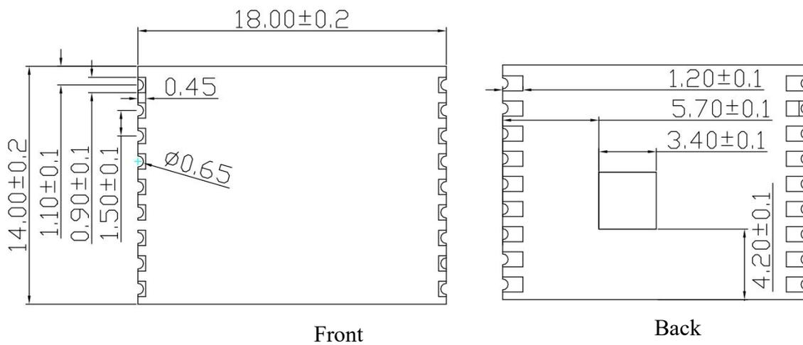
**Figure 4 Dimension diagram**
