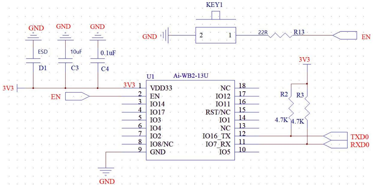
Figure 8 Application circuit diagram
