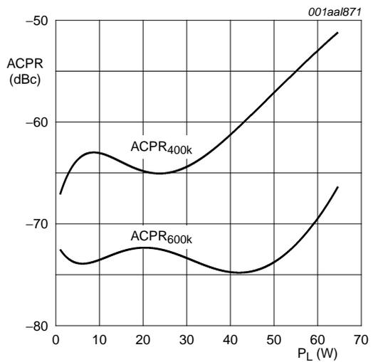
$V_{DS} = 28\text{ V}; I_{DQ} = 550\text{ mA}; f = 1880\text{ MHz}.$
