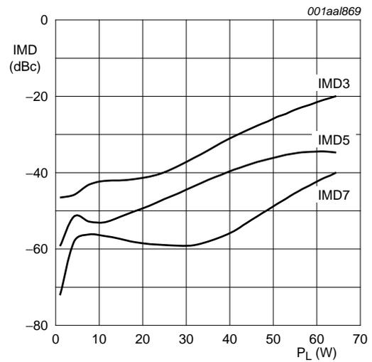
$V_{DS} = 28\text{ V}; I_{DQ} = 550\text{ mA}; f_1 = 1879.95\text{ MHz}; f_2 = 1880.05\text{ MHz}.$
