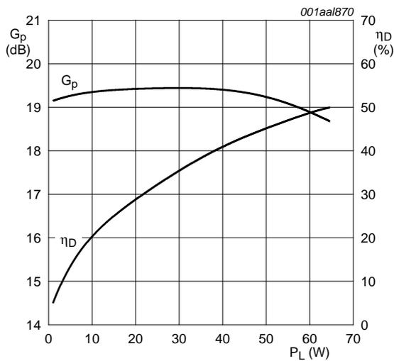
$V_{DS} = 28\text{ V}; I_{DQ} = 550\text{ mA}; f = 1880\text{ MHz}.$
