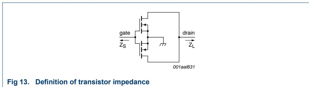
**Fig 13. Definition of transistor impedance**
