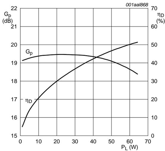
$V_{DS} = 28\text{ V}; I_{DQ} = 550\text{ mA}; f_1 = 1879.95\text{ MHz}; f_2 = 1880.05\text{ MHz}.$
