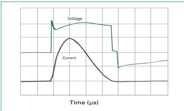
Note: The power dissipation causes a change in avalanche voltage during the surge and the avalanche voltage eventually returns to the original value when the transient has passed.
