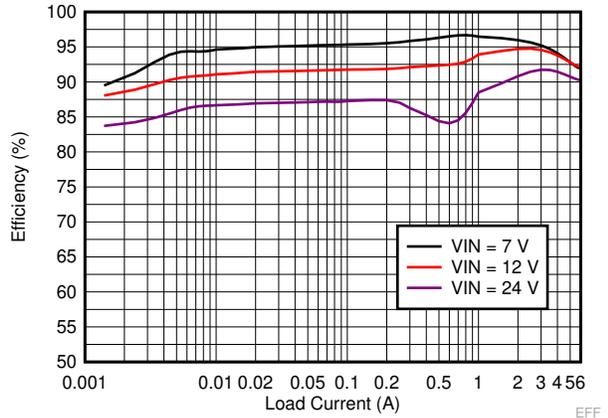
$V_{OUT} = 5\text{ V}$      $f_{SW} = 1000\text{ kHz}$     Auto Mode
