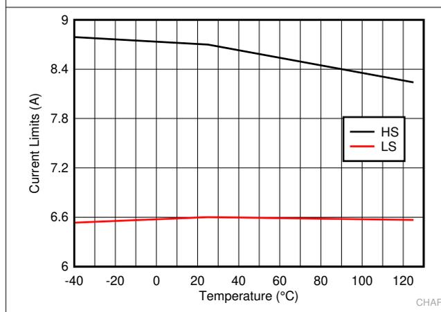
Figure 7-5. LM73605-Q1 High-Side and Low-Side Current Limit
