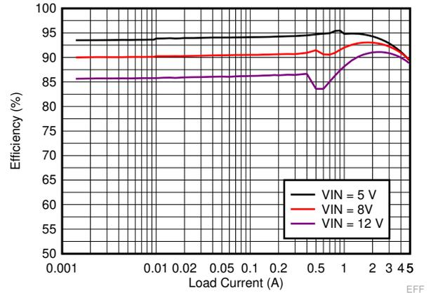
$V_{OUT} = 3.3\text{ V}$   $f_{SW} = 1000\text{ kHz}$  Auto Mode
