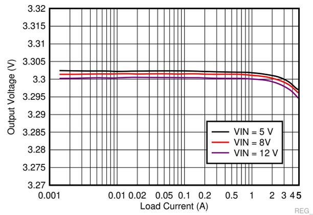
$V_{OUT} = 3.3\text{ V}$      $f_{SW} = 2200\text{ kHz}$     FPWM Mode
