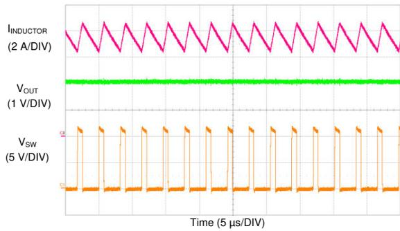
$V_{IN} = 12\text{ V}$        $V_{OUT}$  set at 3.3 V       $f_{SW}$  set at 500 kHz
