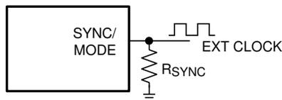
**Figure 8-13. Frequency Synchronization**
