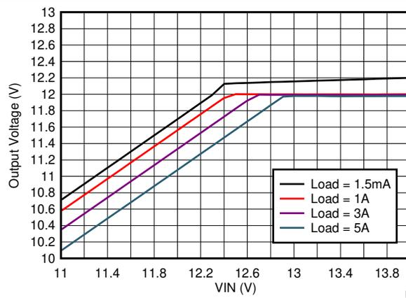
$V_{OUT} = 12\text{ V}$   $f_{SW} = 500\text{ kHz}$  Auto Mode
