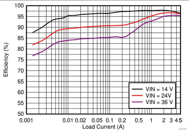
$V_{OUT} = 12\text{ V}$      $f_{SW} = 500\text{ kHz}$     Auto Mode
