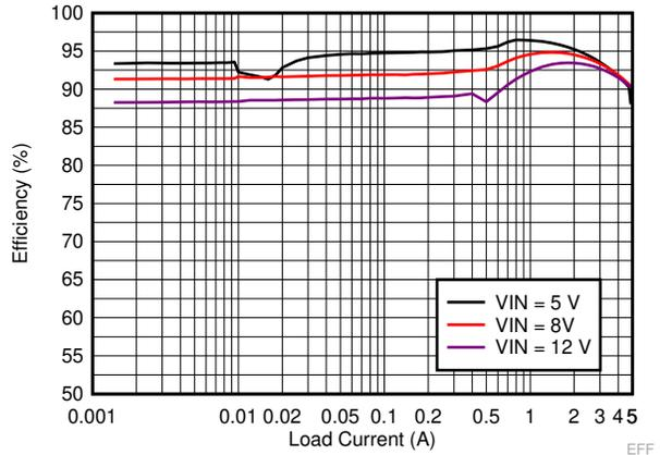
$V_{OUT} = 3.3\text{ V}$   $f_{SW} = 350\text{ kHz}$  Auto Mode
