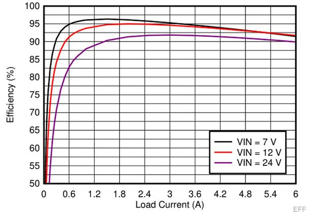
$V_{OUT} = 5\text{ V}$      $f_{SW} = 1000\text{ kHz}$     FPWM Mode
