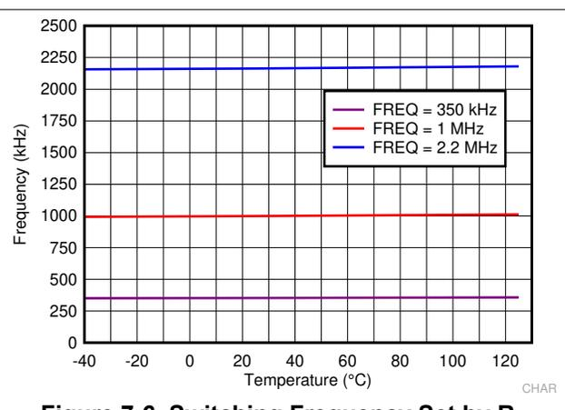
Figure 7-6. Switching Frequency Set by  $R_T$  Resistor
