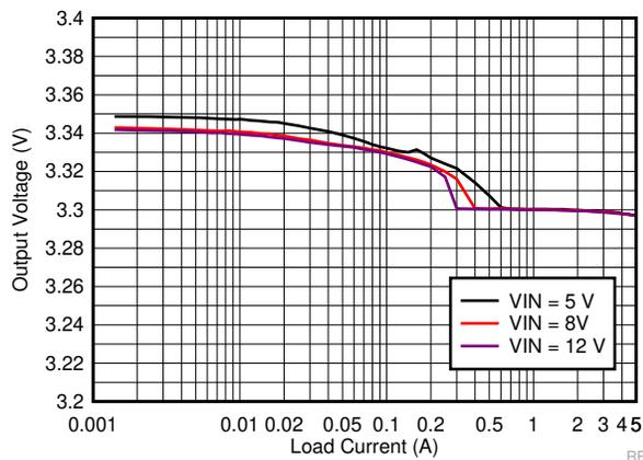
$V_{OUT} = 3.3\text{ V}$      $f_{SW} = 500\text{ kHz}$     Auto Mode
