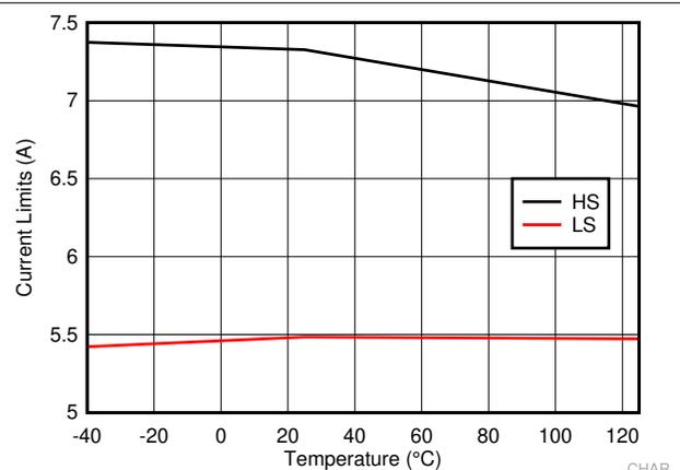
Figure 7-4. LM73605-Q1 High-Side and Low-Side Current Limits
