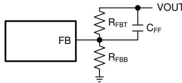
**Figure 8-14. Feedforward Capacitor for Loop Compensation**
