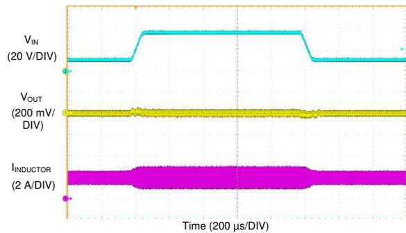
$I_{OUT} = 2\text{ A}$        $V_{OUT} = 3.3\text{ V}$        $f_{SW} = 500\text{ kHz}$
