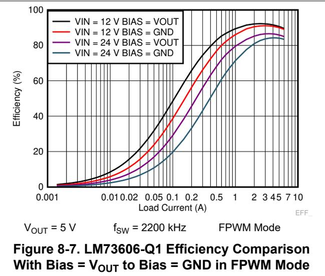
TI recommends tying the BIAS pin to V<sub>OUT</sub> when V<sub>OUT</sub> is equal to or greater than 3.3 V and no greater than 18 V. Tie the BIAS pin to ground when not in use. A ceramic capacitor, C<sub>BIAS</sub>, can be used from the BIAS pin to ground for bypassing. If V<sub>OUT</sub> has high frequency noise or spikes during transients or fault conditions, a resistor (1 to 10 Ω) connected between V<sub>OUT</sub> to BIAS can be used together with C<sub>BIAS</sub> for filtering.
