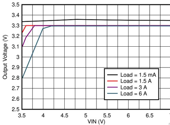
$V_{OUT} = 3.3\text{ V}$   $f_{SW} = 400\text{ kHz}$  Auto Mode
