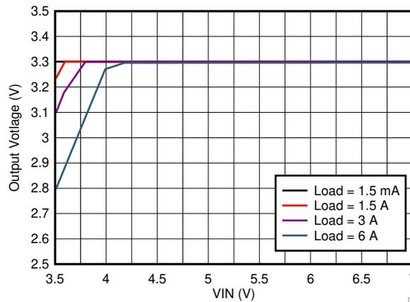
$V_{OUT} = 3.3\text{ V}$   $f_{SW} = 400\text{ kHz}$  FPWM Mode
