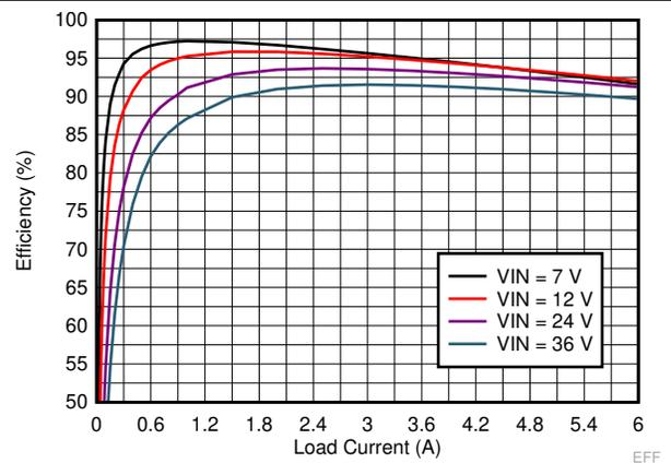
$V_{OUT} = 5\text{ V}$   $f_{SW} = 500\text{ kHz}$  FPWM Mode
