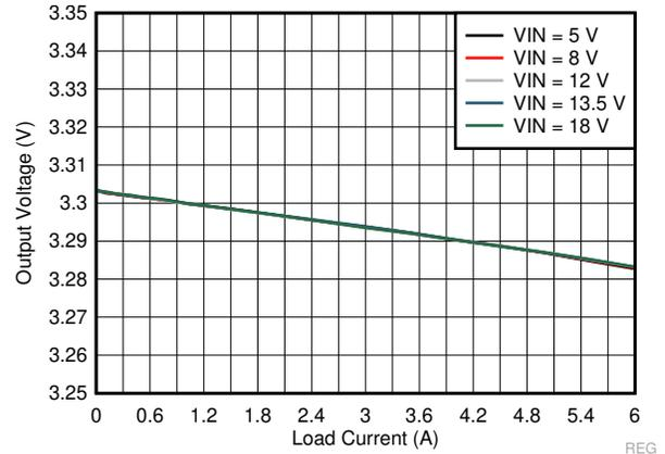
$V_{OUT} = 3.3\text{ V}$      $f_{SW} = 400\text{ kHz}$     FPWM Mode
