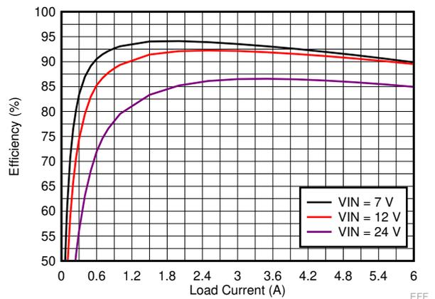
$V_{OUT} = 5\text{ V}$      $f_{SW} = 2200\text{ kHz}$     FPWM Mode
