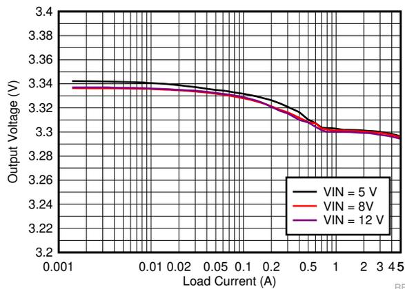
$V_{OUT} = 3.3\text{ V}$      $f_{SW} = 2200\text{ kHz}$     Auto Mode
