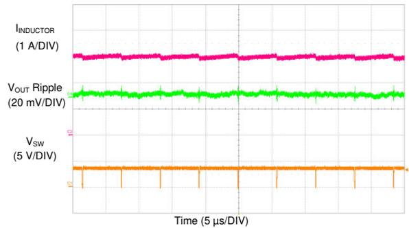
$V_{IN} = 3.66\text{ V}$        $V_{OUT} = 3.3\text{ V}$        $f_{SW}$  set at 500 kHz
