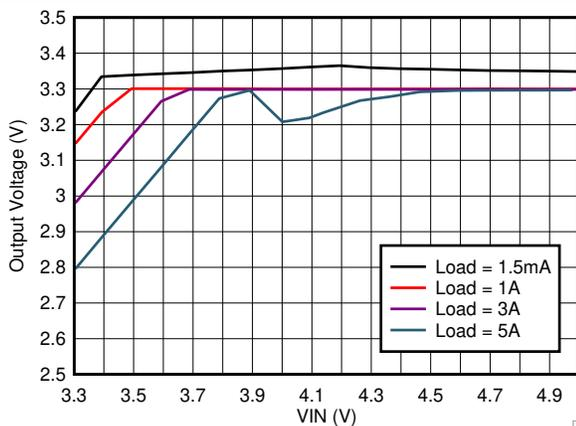
$V_{OUT} = 3.3\text{ V}$   $f_{SW} = 500\text{ kHz}$  Auto Mode
