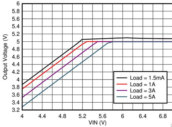
$V_{OUT} = 5\text{ V}$   $f_{SW} = 500\text{ kHz}$  Auto Mode
