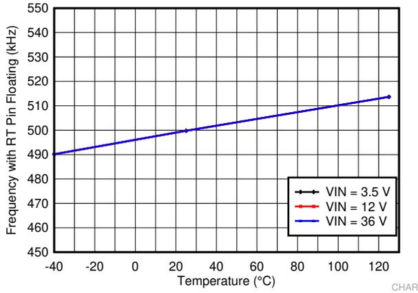
**Figure 7-7. Switching Frequency with RT Pin Open Circuit**
