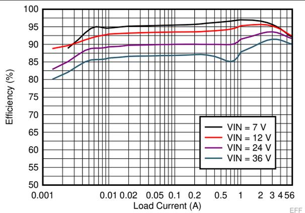
$V_{OUT} = 5\text{ V}$   $f_{SW} = 500\text{ kHz}$  Auto Mode
