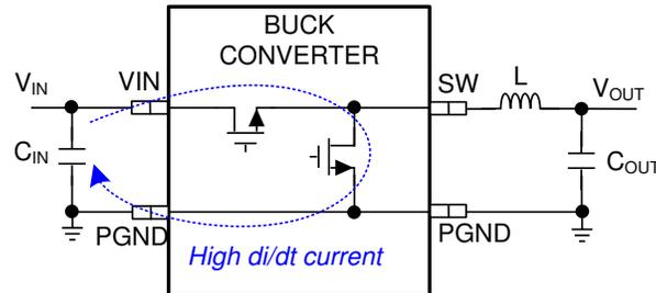
**Figure 9-1. Pulsing Current Path of Buck Converter**
