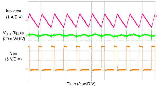
$V_{IN} = 12\text{ V}$        $V_{OUT} = 3.3\text{ V}$        $f_{SW} = 500\text{ kHz}$
