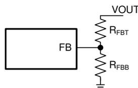
**Figure 8-4. Output Voltage Setting by Resistor Divider**
