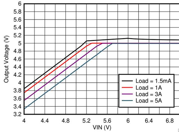
$V_{OUT} = 5\text{ V}$   $f_{SW} = 1000\text{ kHz}$  Auto Mode
