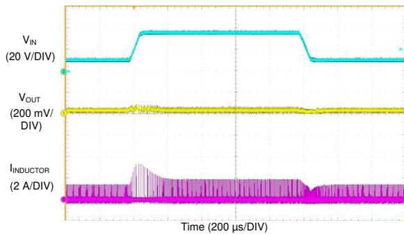
$I_{OUT} = 100\text{ mA}$        $V_{OUT} = 3.3\text{ V}$        $f_{SW} = 500\text{ kHz}$
