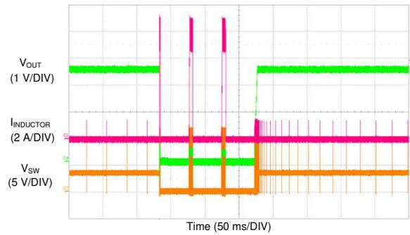
$V_{IN} = 12\text{ V}$        $V_{OUT} = 3.3\text{ V}$        $f_{SW} = 500\text{ kHz}$
