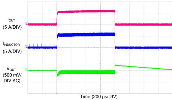
$V_{IN} = 12\text{ V}$        $V_{OUT} = 5\text{ V}$        $f_{SW} = 2200\text{ kHz}$
