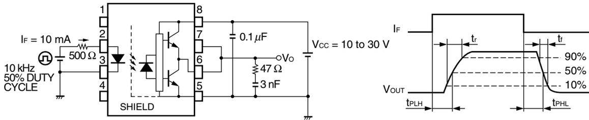
Fig. 7 CMR Test Circuit and Wave Forms
