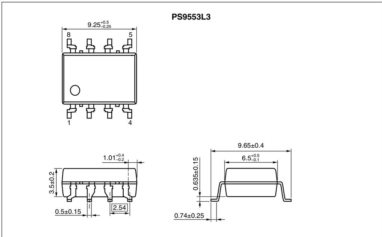
Lead Bending Type For Long Creepage Distance
