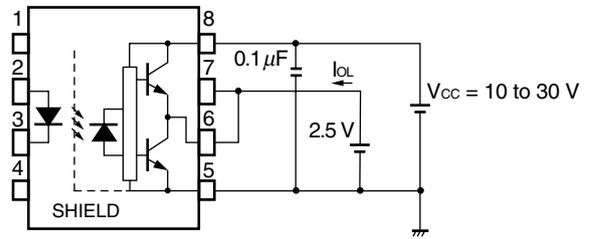
Fig. 3 V<sub>oH</sub> Test Circuit
