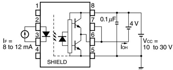
Fig. 2 I<sub>oL</sub> Test Circuit
