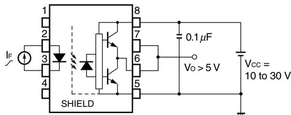
Fig. 6  $t_{PLH}$ ,  $t_{PHL}$ ,  $t_r$ ,  $t_f$  Test Circuit and Wave Forms
