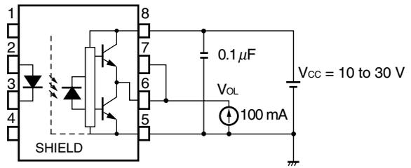
Fig. 5 I<sub>FLH</sub> Test Circuit
