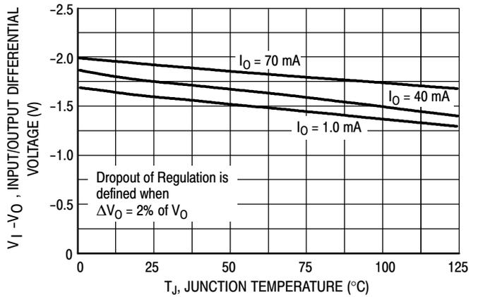
Figure 5. Dropout Voltage versus Junction Temperature
