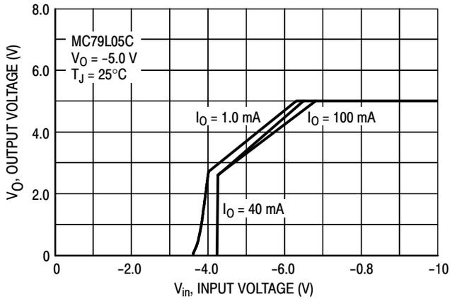
Figure 4. Dropout Characteristics
