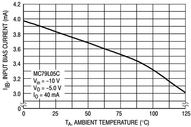
Figure 6. Input Bias Current versus Ambient Temperature
