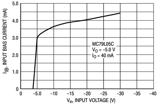
Figure 7. Input Bias Current versus Input Voltage
