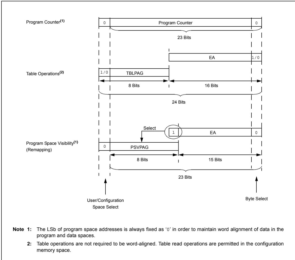
**Note 1:** The LSb of program space addresses is always fixed as '0' in order to maintain word alignment of data in the program and data spaces.
