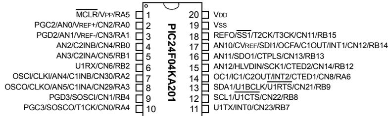
**Note 1:** All device pins have a maximum voltage of 3.6V and are not 5V tolerant.
