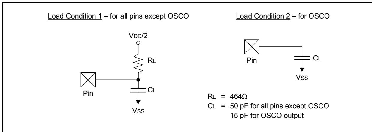
**TABLE 26-18: CAPACITIVE LOADING REQUIREMENTS ON OUTPUT PINS**
