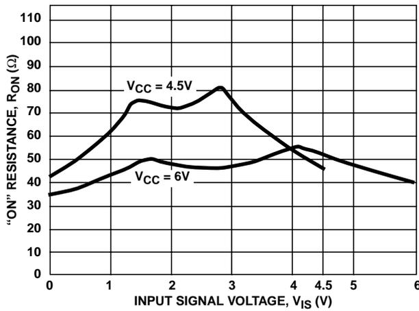
FIGURE 1. TYPICAL "ON" RESISTANCE vs INPUT SIGNAL VOLTAGE
