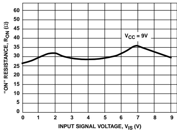
FIGURE 2. TYPICAL "ON" RESISTANCE vs INPUT SIGNAL VOLTAGE
