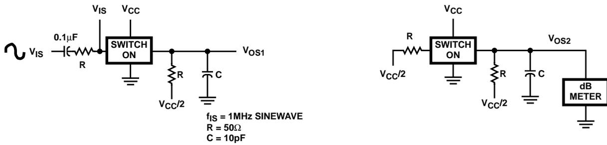
FIGURE 5. CROSSTALK BETWEEN TWO SWITCHES TEST CIRCUIT
