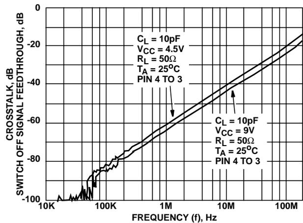
FIGURE 4. SWITCH-OFF SIGNAL FEEDTHROUGH AND CROSSTALK vs FREQUENCY
