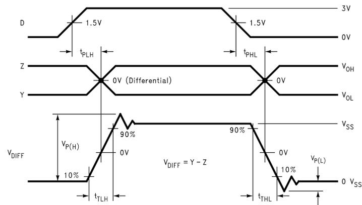
Figure 9. Driver Propagation Delays and Transition Time Waveforms
