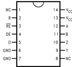
**Figure 1. Connection Diagram
