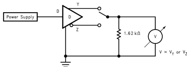
**Figure 6. Differential Driver DC Open Test Circuit**
