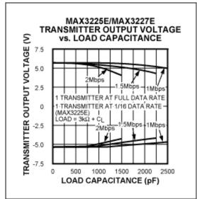
Figure 2sb. MAX3225E transmitter outputs remain compliant with the RS-232 specification, even with a 1Mbit/s data rate and 2000pF load capacitance.
