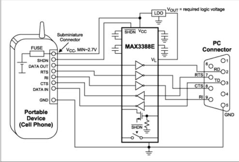
Figure 5. Data-cable designs are simplified by the MAX3388E's programmable logic voltage and a third transmitter, which is used to generate a ring-indicater (RI) signal.
