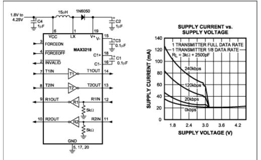
Figure 1. The MAX3218 employs a boost converter followed by a charge pump inverter, and its supply current rises with lower supply voltage.
