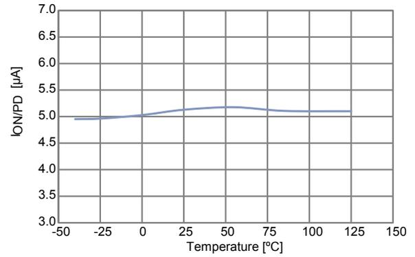
**Figure 20. SS pin bias current vs. temperature**
