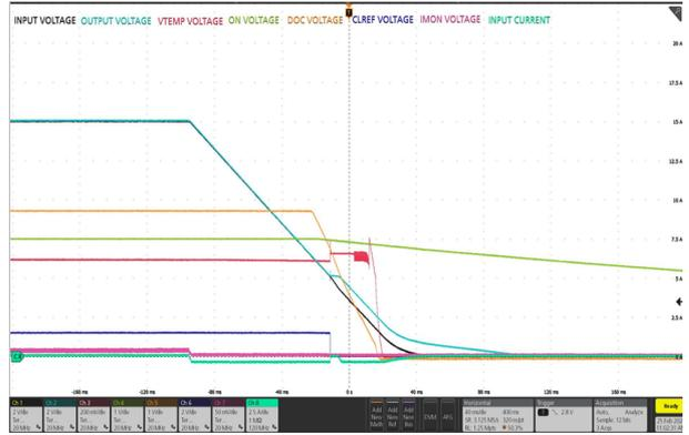
**Figure 26. Startup by  $V_{IN}$  ( $C_{OUT} = 6200\ \mu\text{F}$ , no load)**
