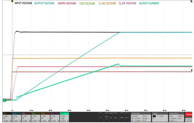
**Figure 28. Startup by ON/PD (no load)**
