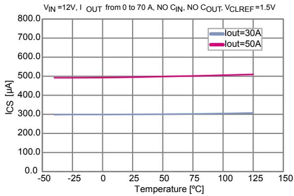
**Figure 13.  $V_{CLREF}$  threshold vs. temperature**
