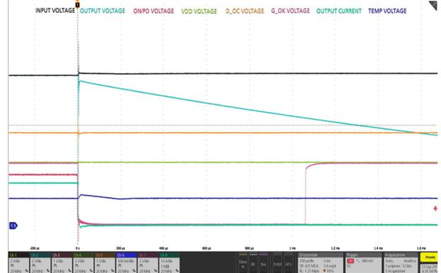
**Figure 32. Startup into output short-circuit**
