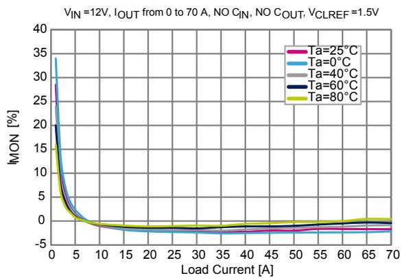
**Figure 11.  $I_{MON}$  current vs. load current**
