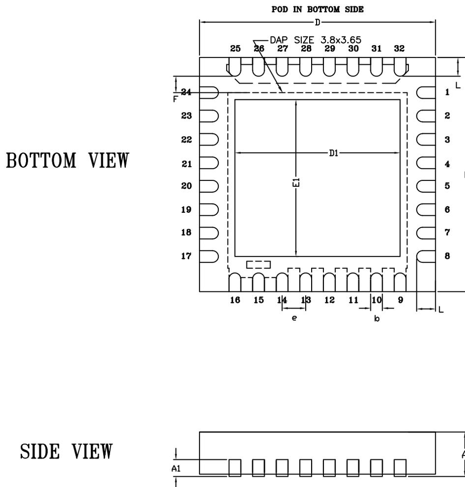
**Table 7. QFN 32 (5 x 5) package mechanical data**
