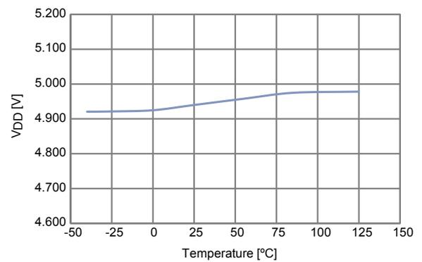
**Figure 16.  $V_{TEMP}$  voltage vs. temperature**
