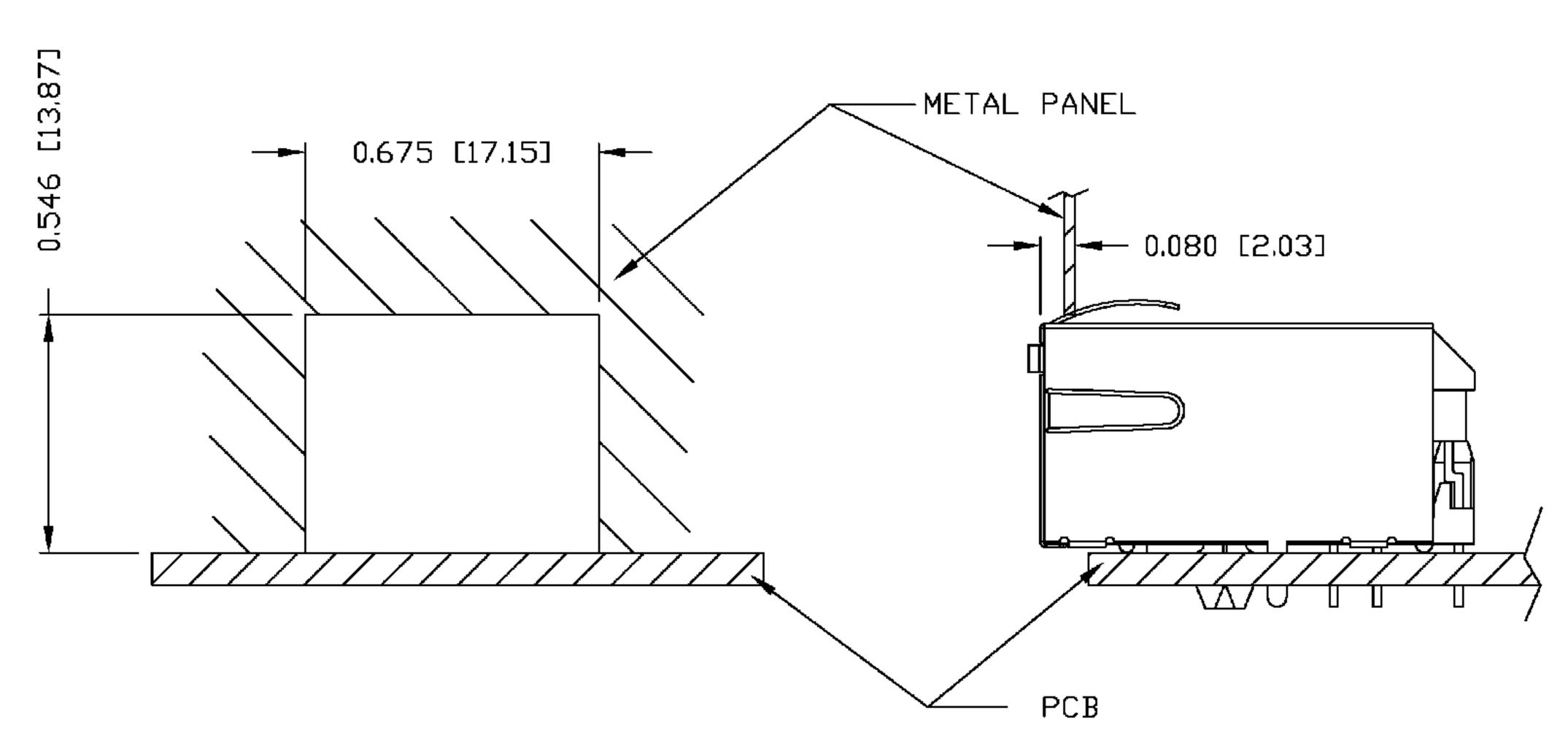
THE DISTANCE OF PANEL INSIDE SURFACE RELATIVE TO FRONT SURFACE OF PART IS ONLY A SUGGESTION. IN CASE THIS DISTANCE IS DIFFERENT, THE REQUIRED PANEL OPENING DIMENSIONS CHANGE ACCORDINGLY.
