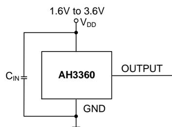
Note: 4.  $C_{IN}$  is for power stabilization and to strengthen the noise immunity, the recommended capacitance is 100nF typical.
