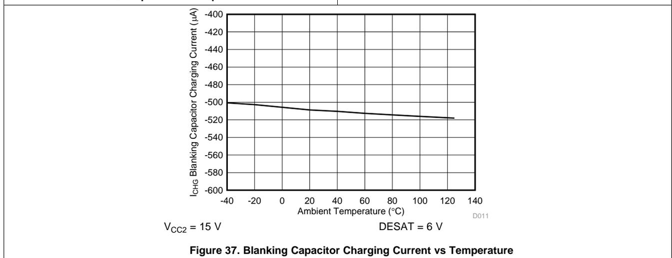
Figure 37. Blanking Capacitor Charging Current vs Temperature
