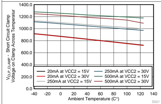
Figure 35.  $V_{CLP\_CLAMP}$  - Short Circuit Clamp Voltage on Clamp Across Temperature
