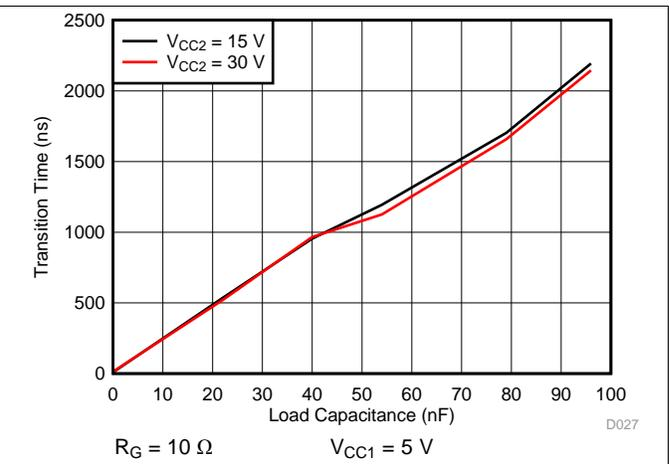
Figure 28.  $t_f$  Fall Time vs Load Capacitance
