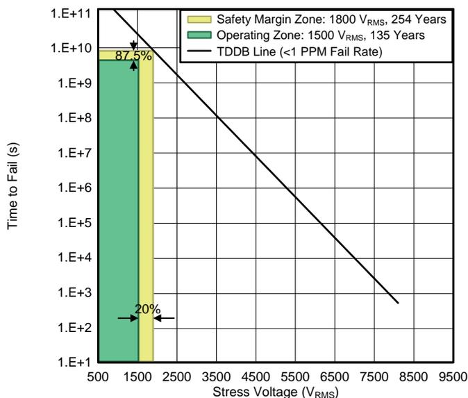
$T_A$  upto 150°C Stress-voltage frequency = 60 Hz
