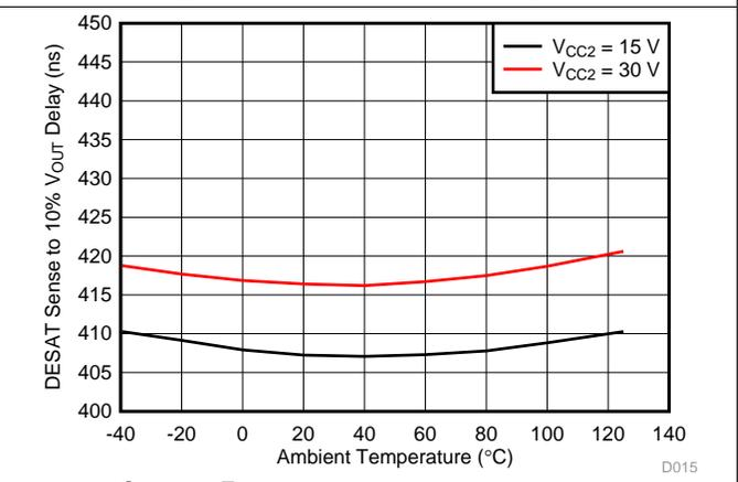
Figure 30. DESAT Sense to  $V_{OUT}$  10% Delay vs Temperature
