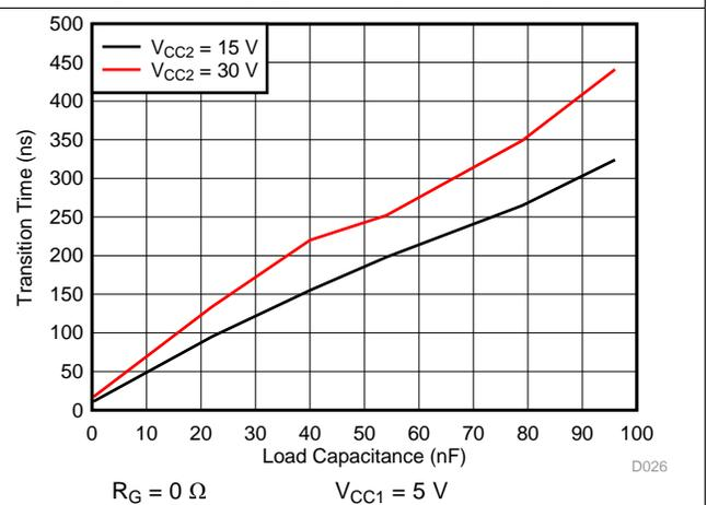
Figure 26.  $t_f$  Fall Time v. Load Capacitance
