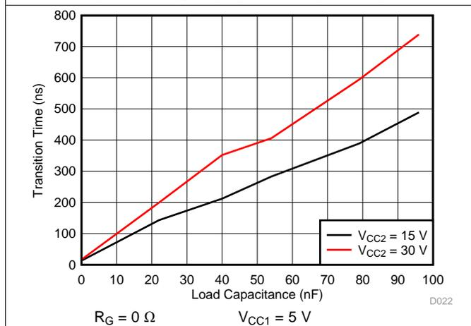
Figure 25.  $t_r$  Rise Time vs Load Capacitance
