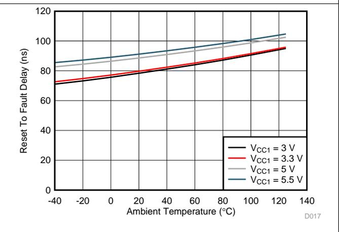
Figure 32. Reset to Fault Delay Across Temperature
