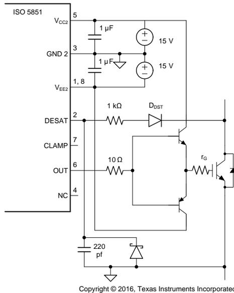
Figure 51. Current Buffer for Increased Drive Current
