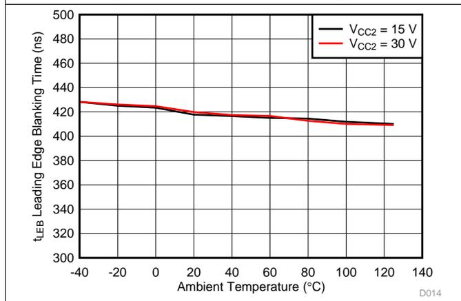
Figure 29. Leading Edge Blanking Time With Temperature
