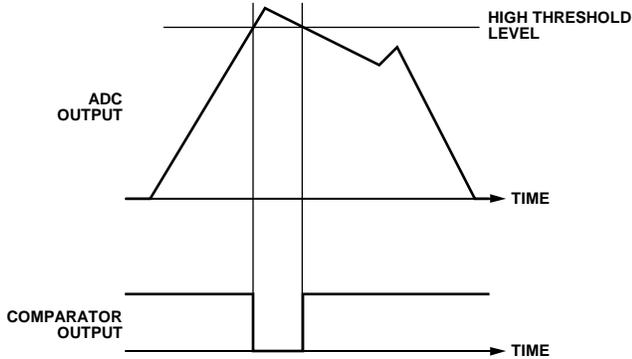
Figure 31. Comparator Behavior in LT Output Mode
