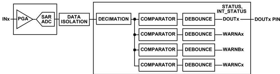
Figure 26. Digital Input Signal Path
