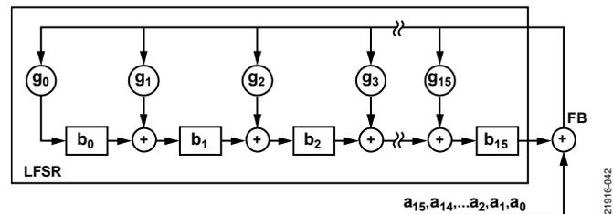
Figure 46. LFSR Generator Used for CRC Calculation
