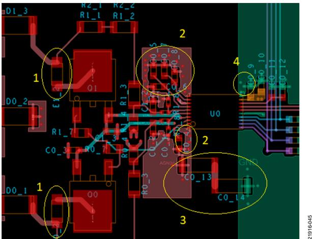
Figure 49. Close Up of the ADE1202 Support Circuitry
