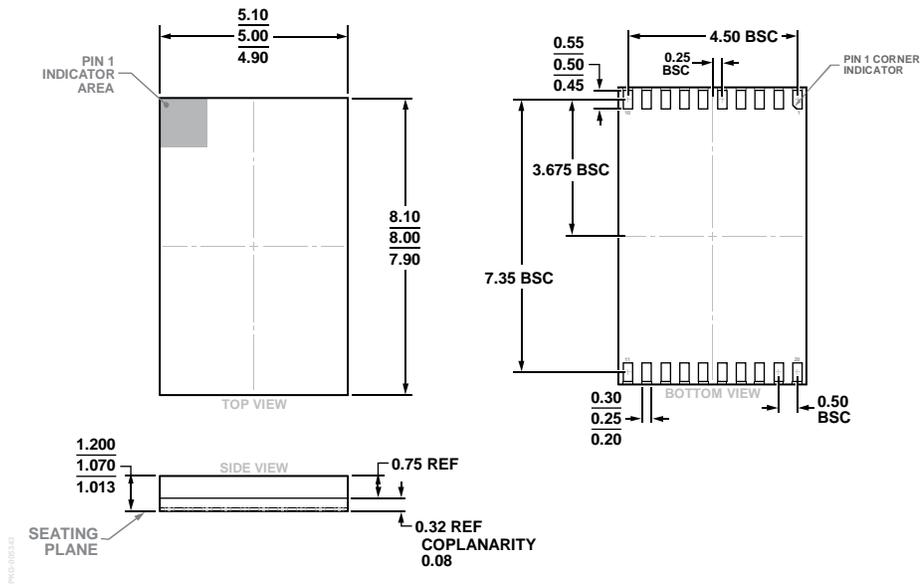
Figure 53. 20-Lead Land Grid Array [LGA] (CC-20-5)
