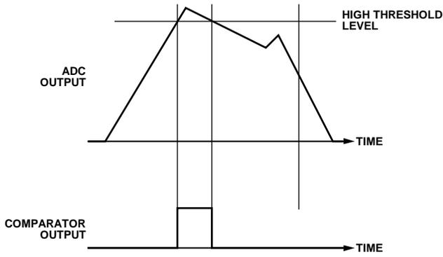
Figure 30. Comparator Behavior in GT Output Mode
