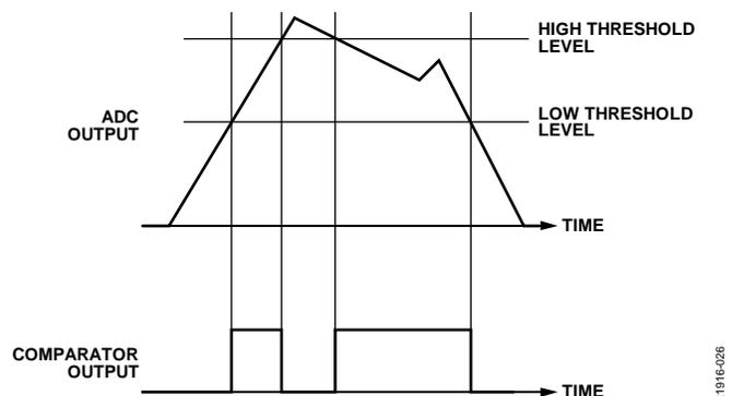
Figure 29. Comparator Behavior in Midrange Output Mode
