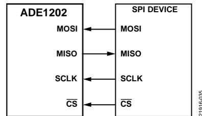
Figure 38. Connecting the SPI to an SPI Device
