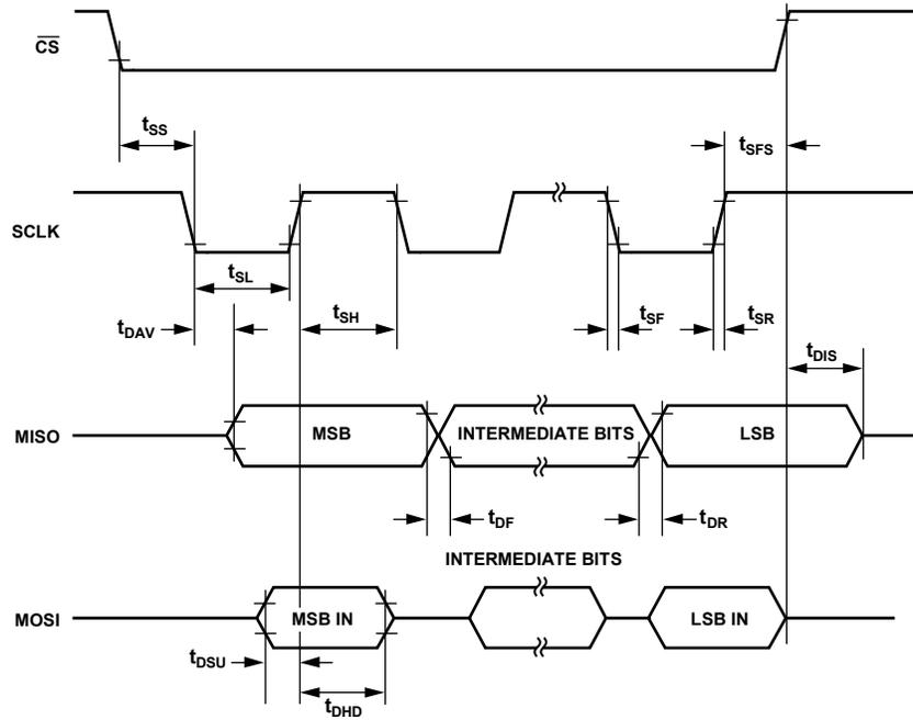
Figure 3. SPI Timing
