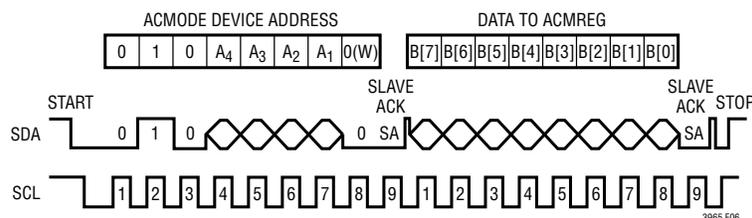
Figure 6. LT3965/LT3965-1 I<sup>2</sup>C Serial Port ACMODE Write Protocol
