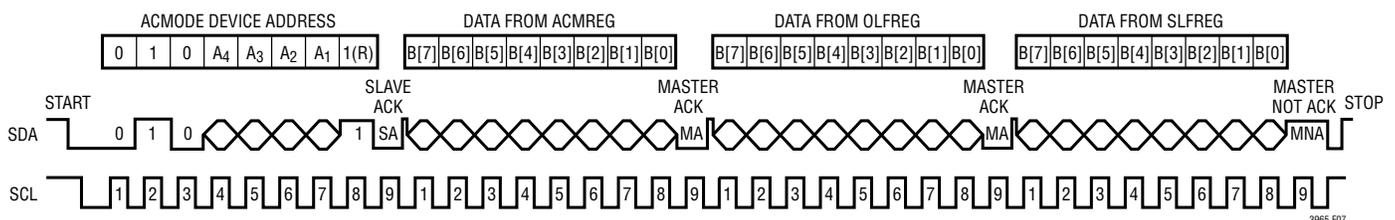
Figure 7. LT3965/LT3965-1 I<sup>2</sup>C Serial Port ACMODE Read Protocol
