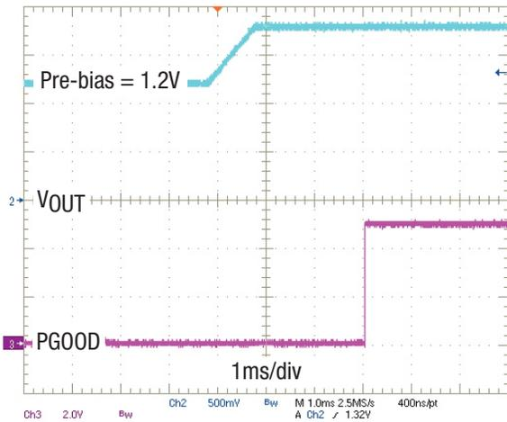
Figure 15. Power-Up with Pre-Bias Voltage,  $I_{OUT} = 0A$
