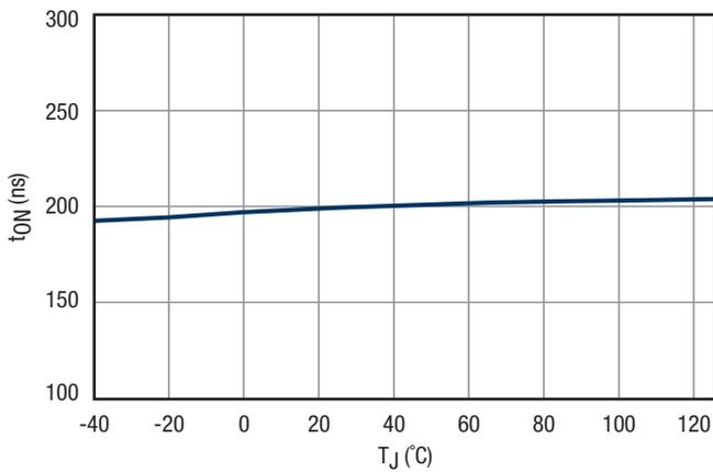
Figure 25.  $t_{ON}$  vs. Temperature,  $R_{ON} = 5.9k$
