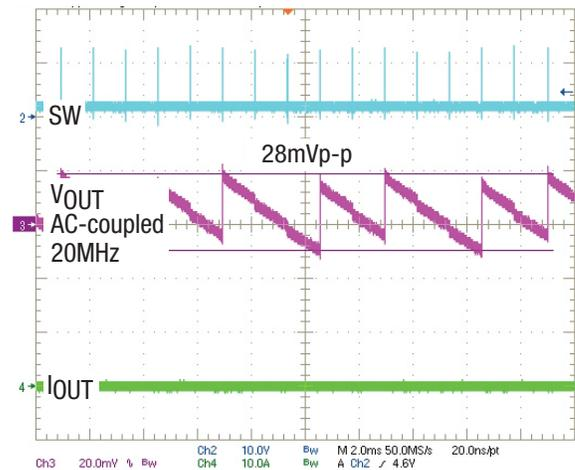
Figure 8. Steady State, DCM,  $I_{OUT} = 0A$
