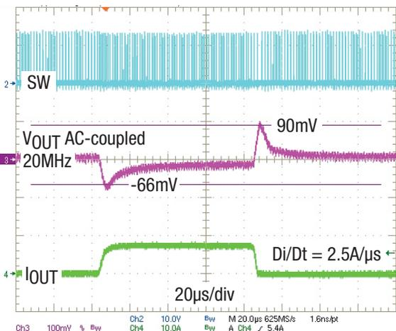
Figure 11. Load Transient, Forced CCM, 0A to 7.5A
