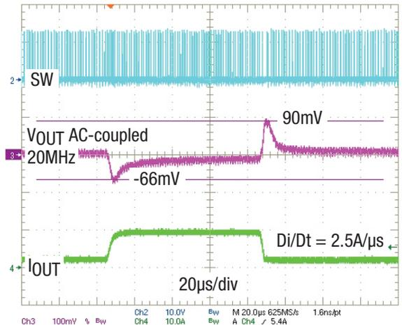
Figure 12. Load Transient, DCM, 2A to 9.5A
