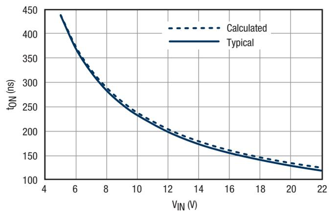
Figure 20.  $t_{ON}$  vs.  $V_{IN}$ ,  $R_{ON} = 5.9k\Omega$
