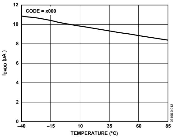
Figure 11. DVDD Supply Current ( $I_{DVDD}$ ) vs. Temperature
