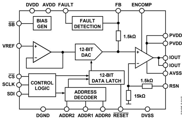
Figure 17. Functional Blocks, Pins, and Internal Connections
