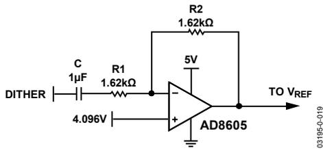
Figure 19. Adding Dither to the Reference Voltage
