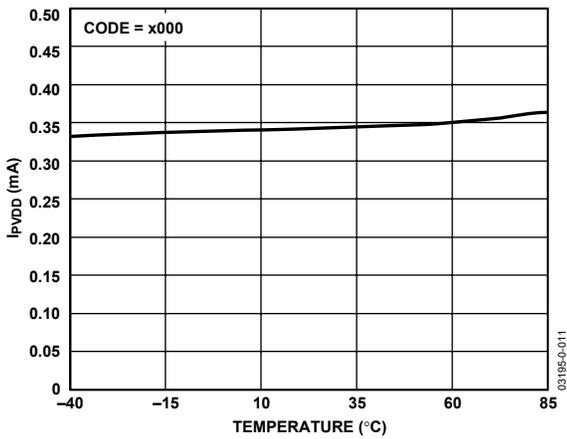
Figure 10. PVDD Supply Current ( $I_{PVDD}$ ) vs. Temperature
