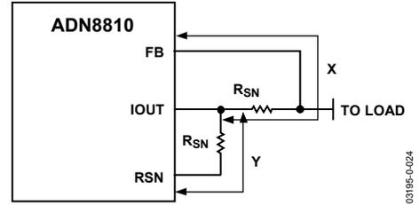
Figure 24. Use Identical Trace Lengths for Sense Resistors
