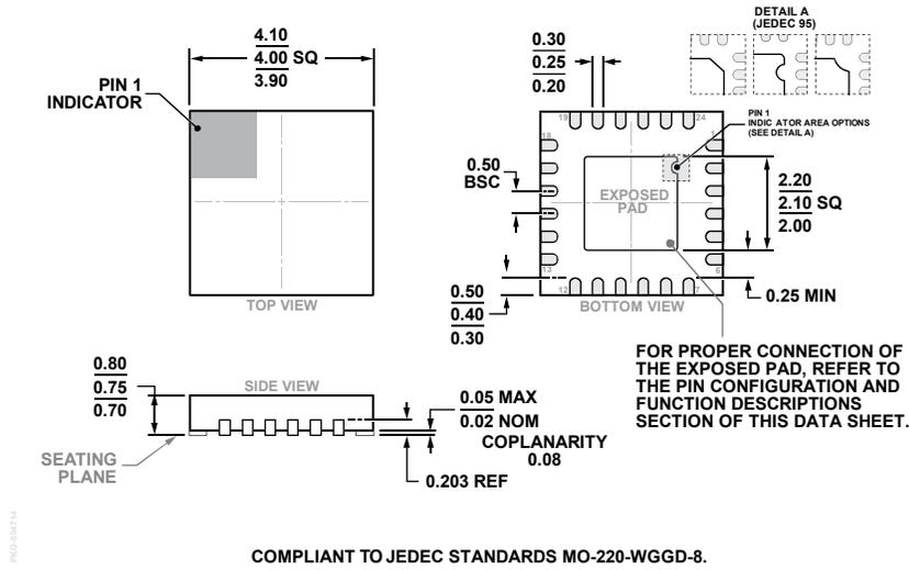
Figure 26. 24-Lead Lead Frame Chip Scale Package [LFCSP]
