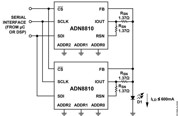
Figure 18. Using Multiple Devices for Additional Output Current
