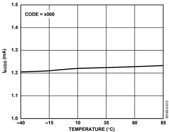
Figure 12. AVDD Supply Current ( $I_{AVDD}$ ) vs. Temperature
