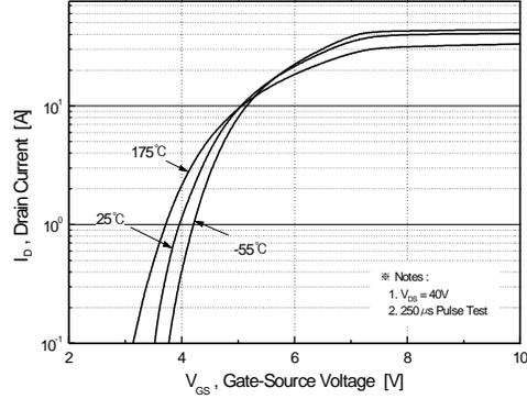
Figure 2. Transfer Characteristics
