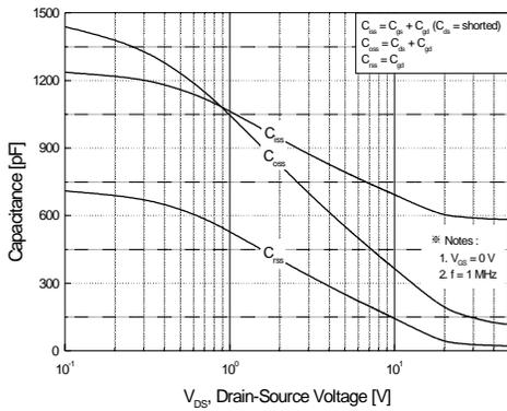
Figure 5. Capacitance Characteristics
