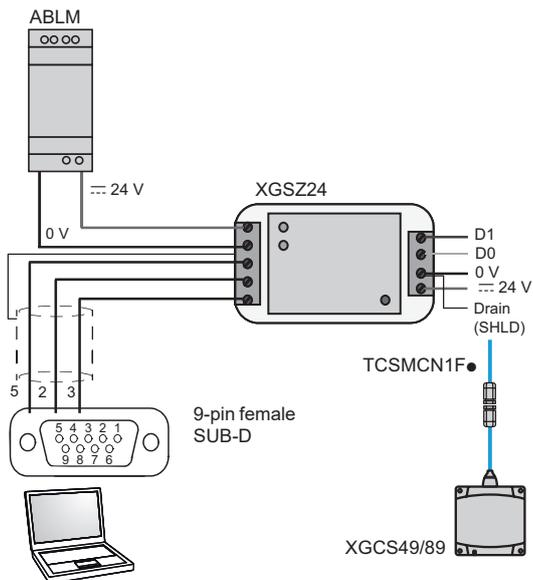
RFID smart antennas can be connected directly to the Modbus port of an automation platform. Up to 15 RFID smart antennas can be linked to the RS 485 port using “T” connectors (in cases where the length of the network exceeds 100 m, fit a line terminator, reference TM7ACTLA). This cabling system is specific to the XG range (powered network). No other Modbus equipment must be connected to it.
