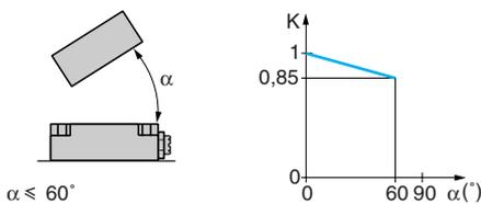
$K$  = correction coefficient to be applied to the nominal sensing distance. Read distance = nominal sensing distance  $\times K$ .
