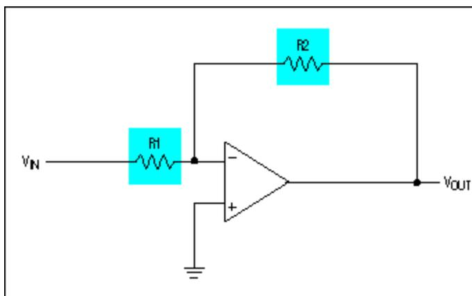
Figure 1. Fixed-gain inverting amplifier.
