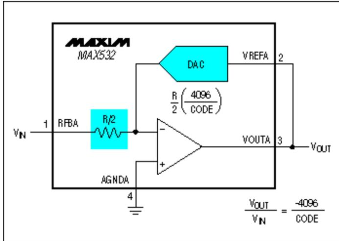
Figure 2. Programmable-gain amplifier.
